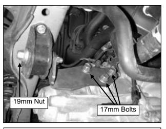
d. Using the supplied bolts and washers, install the AEM<sup>®</sup> engine mount on the transmission, torque the bolts to 61ft-lb. Then replace the factory washers and nut on the mounting stud.
