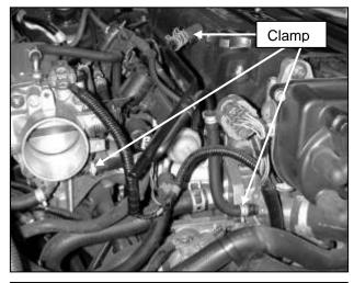
c. CAUTION: Ensure the engine is completely cool before removing the coolant hose, or hot coolant will escape from the cooling system and cause injury or damage. Be sure to capture any lost coolant in a clean container. Remove the clamps securing the cam cover breather tube and coolant circulation tube, and remove it.
