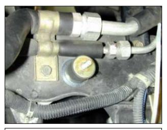
f. Install the supplied  $\frac{1}{4}$ " spacer and rubber mount over the threaded hole located near the A/C line behind the passenger headlight. The  $\frac{1}{4}$ " spacer should sit between the rubber mount and the body of the vehicle.
