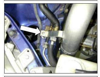
h. The intake pipe's mounting bracket will line up with the rubber mount installed earlier. Use the supplied serrated nut and washer to secure in place. See the diagram below for proper installation of the rubber mount.
