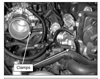
d. Attach the supplied 5/16" hose onto the coolant outlets using 2 of the supplied ¾" clamps to secure the hose in place. **NOTE: Replace any coolant recovered during hose removal by replenishing the recovery tank**.
