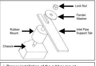
i. Proper installation of the rubber mount assembly.
