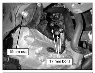
a. Using a 19mm socket, remove the engine mount nut. Also remove the three 17mm bolts and remove the mount.
