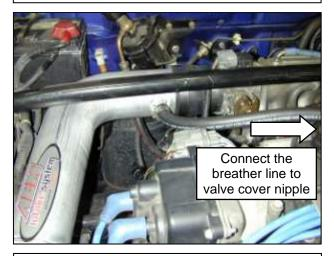
g. Install the AEM<sup>®</sup> inlet pipe into the vehicle and secure to the throttle body using a #48 hose clamp. Attach the supplied breather hose to the intake pipe's nipple; connect the opposite end to the valve cover's inlet. Secure each end of the breather hose in place with the two supplied hose clamps.
