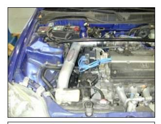
AEM<sup>®</sup> intake system installed
