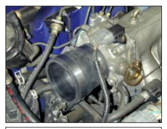
e. Install the reducing coupler onto the throttle body and secure using the #44 hose clamp.
