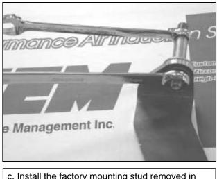
c. Install the factory mounting stud removed in step #3b through the supplied engine mount bracket. Secure in place with the provided nylock nut and washer.
