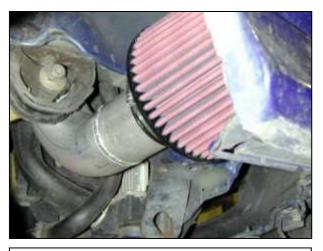
j. Install the AEM<sup>®</sup> air filter onto the inlet pipe. Once proper fitment is achieved, secure the air filter in place with the supplied hose clamp.
