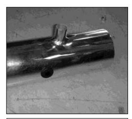
c. Install the supplied grommet into the intake pipe as shown.
