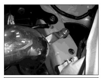
g. Use the supplied washer and nut to secure the intake pipe's bracket in place. Refer to the diagram for proper installation of the rubber mount assembly.
