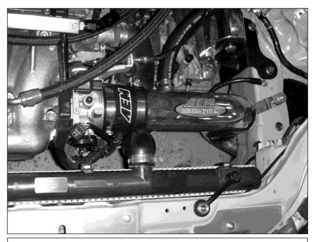
j. Position the intake pipe assembly in the engine bay so that it does not make contact with vehicle. When proper fitment is achieved, tighten all hose clamps and the nut on the rubber mount.
