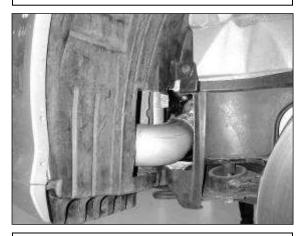
q. The fender liner must be trimmed for the intake system to fit properly.
