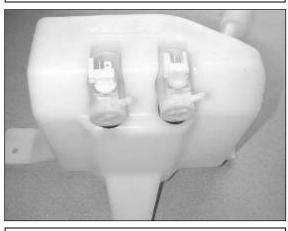
e. Reinstall the two pump grommets and the fill tube grommet on the replacement washer bottle. Wet the grommets with soapy water and insert the two washer pumps and fill tube.
