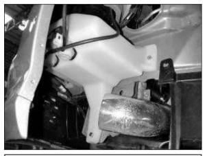
f. Secure the new washer bottle with the three air box bracket bolts removed in step 2n. Reconnect the two feeder lines and the two electrical connectors to the pumps.
