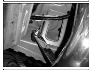
g. Secure the mounting bracket to the rubber mount with the supplied washer and nyloc nut.
