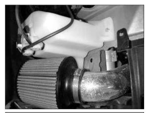
i. Install the AEM<sup>®</sup> air filter onto the lower end of the intake pipe.
