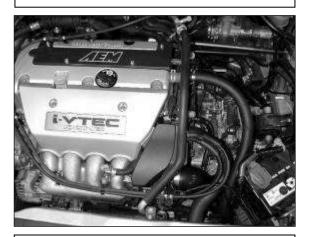
AEM<sup>®</sup> intake system installed.
