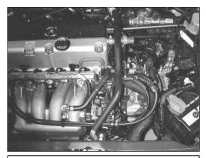
I. Factory air box system removed from vehicle.
