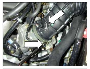
a. Loosen the clamp around the throttle body using a 5.5mm socket or screwdriver. Pull the Intake Air Temperature (IAT) sensor out of the intake tube by loosening the spring loaded clamp.
