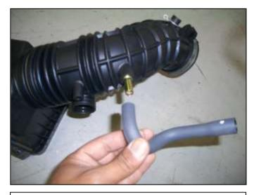
g. Remove the small hose from the factory intake system.
