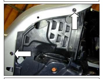
i. From underneath the vehicle, remove the fasteners shown in the picture.
