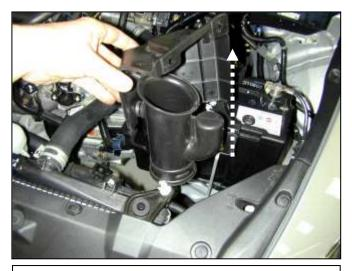
g. Pull upward on the plastic cover to remove the resonator box / intake tube.
