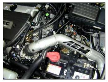
d. Insert the AEM<sup>®</sup> intake pipe into the engine bay. Line up the bracket of the intake pipe with the rubber mount while also inserting the intake pipe into the coupler on the throttle body.
