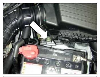
c. Remove the airbox mounting bolt shown in the picture.
