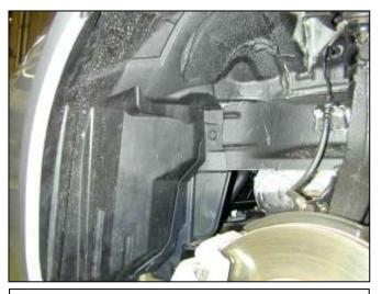
h. Remove the fasteners securing the driver-side wheel well liner.
