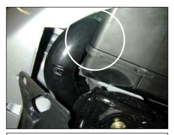
n. Reach up inside the space in front of the resonator assembly with a 10mm socket or wrench and remove the other mounting bolt.
