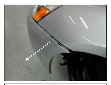
m. Unsnap the corner of the bumper cover as shown in the picture. This will help in the removal of the resonator assembly.
