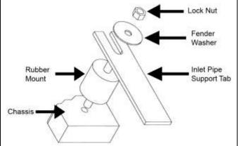
Proper installation of the rubber mount assembly.
