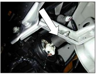
c. Install the rubber mount in the bracket behind the front left headlight as shown in the picture. Secure it in place with a washer and Nylock nut as shown.
