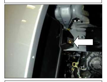
k. Remove the resonator mounting bolt shown in the picture.
