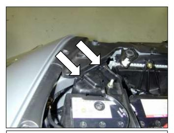
f. Remove the two fasteners securing the plastic cover in front of the battery.
