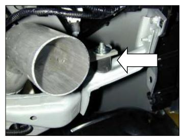
f. Install a nut and washer to secure the intake bracket to the rubber mount as shown. Ensure the rubber mount assembly is properly installed, see diagram for reference.
