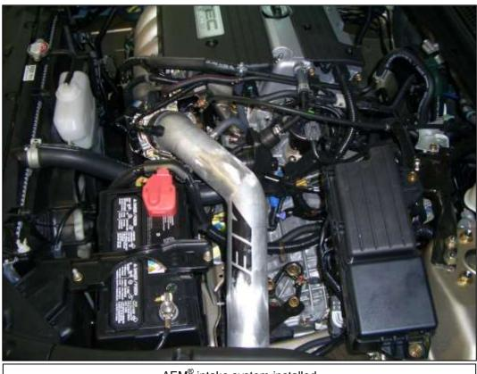
AEM<sup>®</sup> intake system installed
