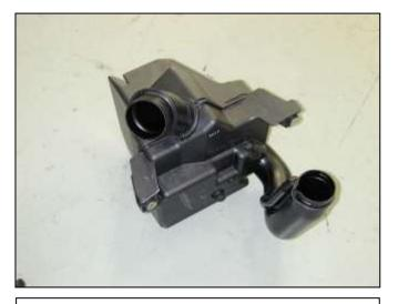
o. Remove the resonator assembly from the vehicle.
