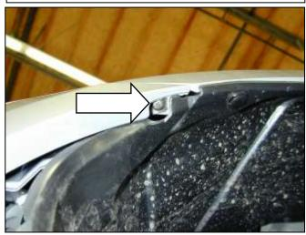
I. Remove the screw holding the corner of the front bumper cover.
