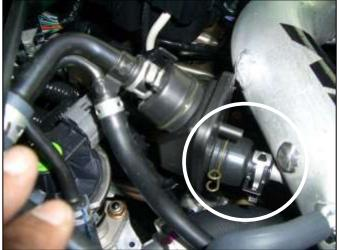
j. Attach the oil trap coupler to the oil trap and secure with the stock clamp. Attach the small end to the intake pipe and secure with provided spring clamp. NOTE: This intake system is designed to use the factory oil trap, failure to use the oil trap will result in poor performance and possible engine damage may result.
