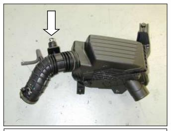
e. Carefully remove the airbox assembly from the engine bay. Remove the oil trap from the inlet duct and retain the clamps for later use.
