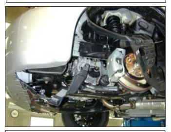
j. Tuck the fender liner out of the way behind the brake rotor.
