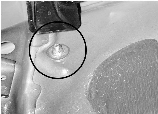
e) Secure the rubber mount using the supplied washer and nylok nut.
