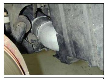
I. Trim inner fender liner and under tray as shown for proper fit.
