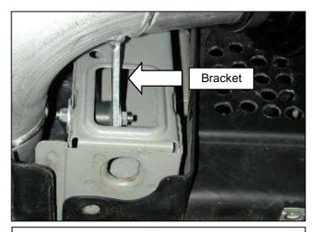
i. Install the lower intake pipe behind the radiator with the bracket sliding onto the rubber mount. Use the washer and screw on the nylok nut but do not tighten at this time.
