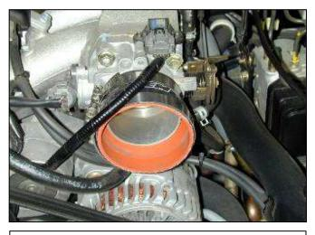
d. Install the 3.00"-3.25" reducing coupler on to the throttle body using the #44 hose clamp. Ensure that the inside of the AEM<sup>®</sup> intake pipes and air filter are clean and free from any foreign objects and/or obstructions.
