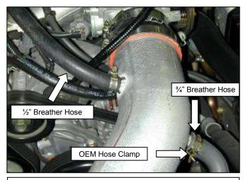
f. Install the upper intake pipe by inserting the end with the  $\frac{1}{2}$ " nipple into the 3.25" side of the coupler on the throttle body. Attach the  $\frac{1}{2}$ " breather hose and the  $\frac{3}{4}$ " factory breather hose as shown. Use the factory hose clamp on the  $\frac{3}{4}$ " hose and the supplied hose clamp on the  $\frac{1}{2}$ " hose.
