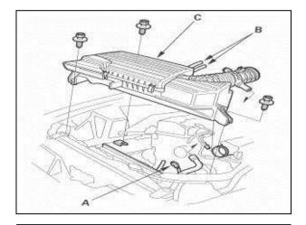
b. Disconnect the Air Control Solenoid Valve Connector (A) and then remove the vacuum hoses (B).
