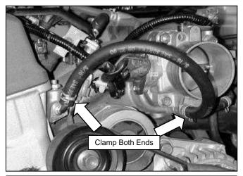
b. Install the provided 5/16" hose between the throttle body and the bleeder outlet vacated by the removal of lower hose of the metal tube loom. Use the factory hose clamps as shown. **NOTE: Replace any coolant recovered during hose removal by replenishing the recovery tank.**
