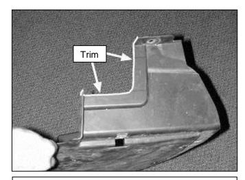
m. Trim the passenger side under tray as shown to provide cooler air to the air filter element. Install the under tray, trimming or notching them for tube clearance where required.
