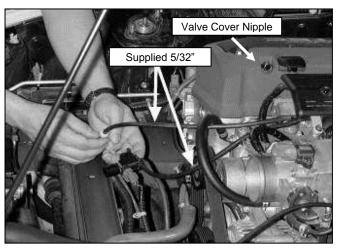
c. Replace the factory Air Control Solenoid Valve vacuum lines with the supplied 5/32" lines, as shown. Use the two supplied zip ties to zip tie the hoses away from the serpentine belt. Install the supplied breather hose onto the valve cover nipple using the supplied hose clamps.
