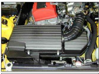
Factory air box system installed
