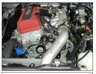
o. Ensure the air filter is not touching any part of the vehicle. Position the inlet pipe for best fitment. Be sure that the intake pipe or any other component is not in contact with any part of the vehicle. Tighten the hose clamps at the throttle body and silicone coupling. Tighten the nut on the mounting bracket. Check for proper hood clearance. Re-adjust pipe if necessary.
