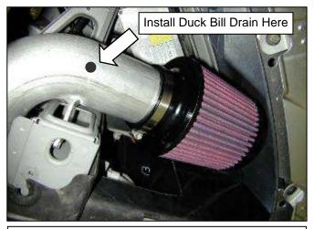
n. Install the AEM<sup>®</sup> air filter onto the end of the intake pipe. Push the air filter over the inlet pipe until the stop in the air filter is reached. Then install one hose clamp to secure the air filter onto the inlet pipe. Once fitment is checked, tighten the hose clamp.
