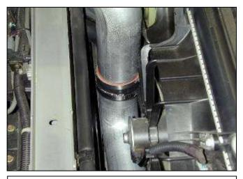
j. Using the 3.25" silicone hose and two #48 hose clamps supplied, attach the upper and lower intake pipes together.
