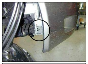
g. Install the supplied rubber mount into the passenger side radiator support frame rail as shown. When tightening the nut, tighten until the thin outer wall of the support starts to deflect (See step 3h for a closer view).
