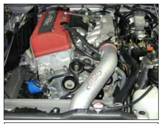
AEM<sup>®</sup> intake system installed
