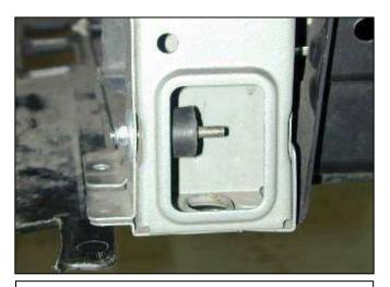
h. Install the supplied rubber mount into the passenger side radiator support frame rail as shown. When tightening the nut, tighten until the thin outer wall of the support starts to deflect.
