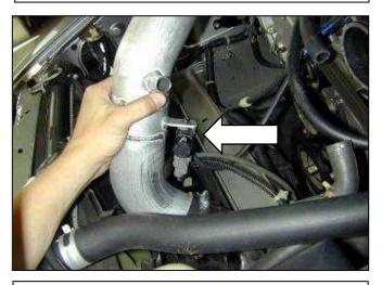
e. Using the factory bolt, secure the Air Control Solenoid Valve to the bracket on the upper intake pipe as shown.
