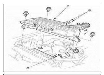
c. Loosen the throttle body hose clamp, loosen the three mounting bolts, and remove the air cleaner housing/intake duct (C) assembly.
