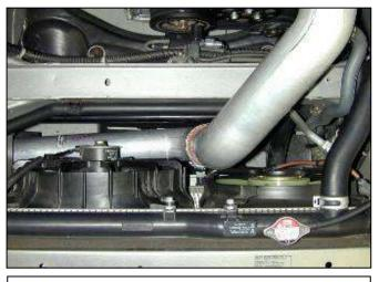
k. Ensure there is sufficient clearance between the lower intake pipe and radiator fan guard, the A/C line, and the sway bar.
