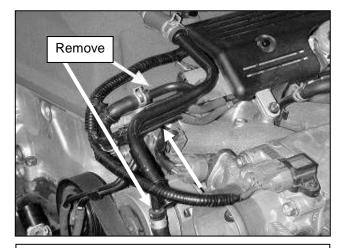
e. CAUTION: Ensure the engine is completely cool before removing the coolant hose, or hot coolant will escape from the cooling system and cause injury or damage. Be sure to capture any lost coolant in a clean container. Remove the metal tubing loom, which will include the breather hose, coolant hose and air control solenoid valve vacuum hoses. Make sure to note proper hose routing (Place the clean catch container under the loom, as coolant will leak from the lower hose).
