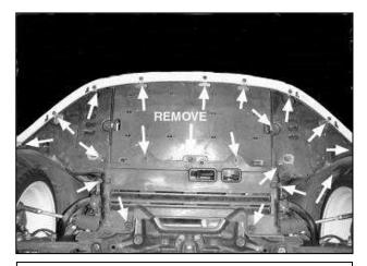
d. Raise the front of the vehicle with a jack. Refer to your owner's manual for proper jack and jack stand placement to properly support vehicle. Support your vehicle using properly rated jack stands before wheel removal or while working under the vehicle.
