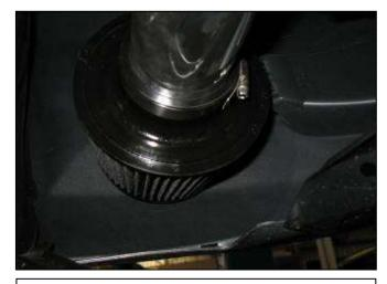
I. From under the vehicle, install the AEM<sup>®</sup> Dryflow<sup>™</sup> air filter onto the end of the lower pipe. Push the air filter onto the intake pipe until the stop inside is reached. Then secure the air filter using a #48 hose clamp.
