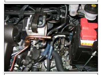
h. Remove the air filter housing and resonator from the vehicle by sliding the resonator off the throttle body and lifting straight out.
