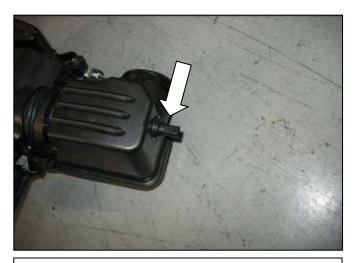
p. Carefully remove the IAT sensor from the previously removed resonator and air filter housing.
