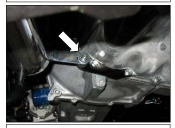
k. With the intake pipe bracket aligned with the rubber mount, install a washer and serrated nut to secure.
