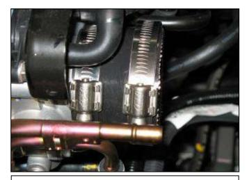
f. Install the supplied reducing coupler onto the throttle body using a #40 and a #44 hose clamp as shown.
