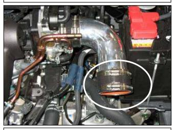
h. Install the straight coupler onto the end of the upper pipe and secure using two #44 hose clamps.
