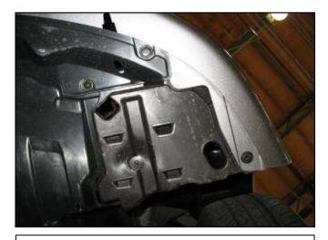
j. Remove the retaining clips and bolts securing the driver side splash shield to the bumper and chassis.
