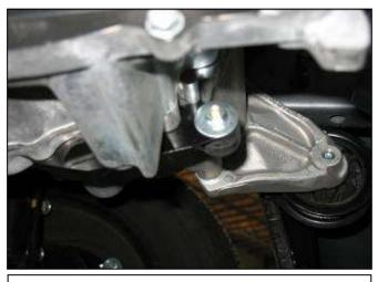
c. Install the supplied rubber mount into the previously installed transmission bracket using a flat washer and serrated nut. The rubber mount should face the driver's side.
