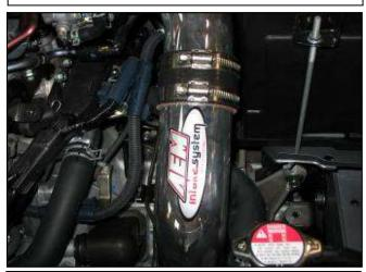
j. From under the vehicle, slide the lower intake pipe up and into the previously installed coupler. Align the bracket with the rubber mount installed in step 3c.
