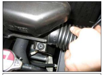
g. Remove the air inlet hose from the air filter housing by sliding off the housing.
