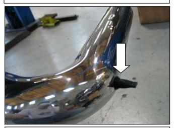
i. Locate the hole on the lower intake pipe and insert the supplied duck bill drain as shown.
