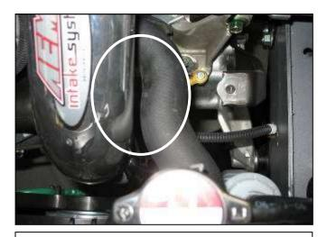
m. Check for clearance around the lower pipe. If the radiator hose is too close or touching, gently bend its support bracket for clearance. Once clearance has been verified, tighten all hose clamps and the nut on the rubber mount.
