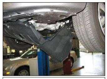
m. Unclip the underbody tray from the driver's side fender liner and let it hang to gain access behind the front bumper as shown.
