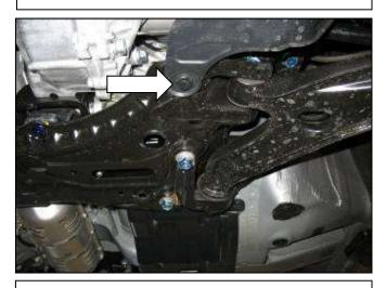
I. From underneith the vehicle remove the plastic retaining clip located on the driver's side subframe.
