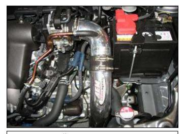
AEM® intake system installed
