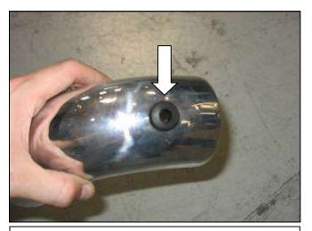
d. Install the rubber grommet into the hole on the short upper pipe as shown.
