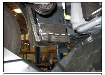
n. From underneith the vehicle, trim the driver's side fender liner to allow clearance.
