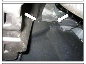
k. From inside the wheel well, remove the retaining clips securing the underbody tray to the chassis.
