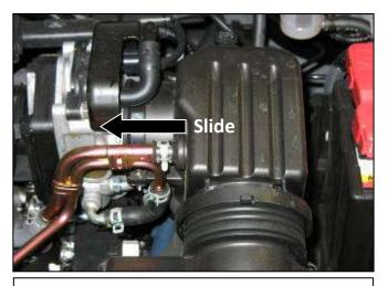
d. Remove the metal breather hose from the upper resonator by compressing the clamp and pulling the hose out of the resonator.
