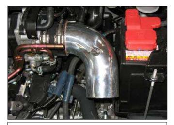
g. Slide the short upper intake pipe into the throttle body with the IAT sensor facing the firewall. If clearance is needed, loosen the battery mount and slide battery away from pipe.
