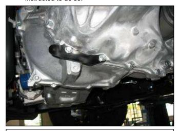
b. Install the transmission bracket using the two bolts removed in step 2q. with the third hole towards the front of the vehicle as shown. Torque bolts to 33 ft-lbs.
