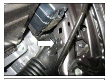
i. Remove the air inlet hose from the chassis by removing the plastic retaining clip securing it and pulling it out of the fender opening.
