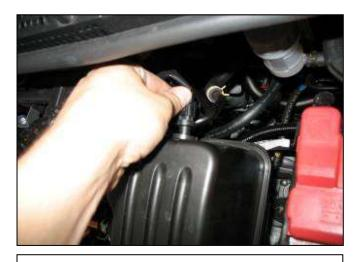
b. Unplug the Inlet Air Temperature (IAT) sensor from the wiring harness on the back side of the resonator as shown.
