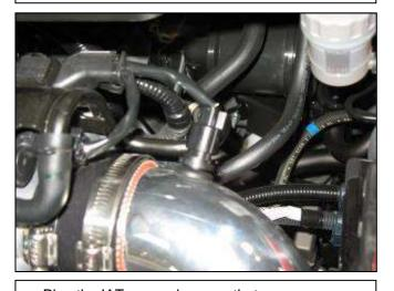
n. Plug the IAT sensor harness that was disconnected in step 2b into the installed sensor on the upper intake pipe.
