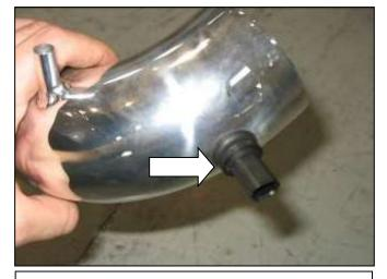
e. Carefully install the IAT sensor into the grommet. Fitment may be tight, if so use soapy water to ease installation.
