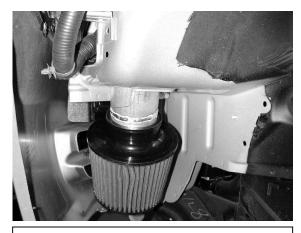
j. Install the air filter and secure in place using the supplied hose clamp.
