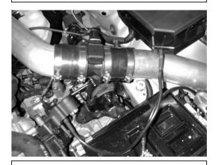
h. Install the second 3" coupler onto the lower intake pipe and secure in place using the supplied 3" hose clamps. Install the washer and nyloc nut to secure the inlet pipe bracket to the rubber mount. Failure to install the rubber mount will void all warranties of the Cold Air System.
