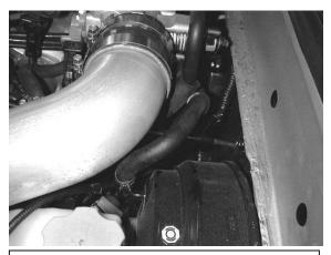
e. Remove the brake booster vacuum line hose clamp and push the vacuum hose down completely over the metal nipple and re-install hose clamp to make clearance room for the intake pipe.
