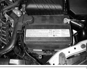
b. Disconnect and remove the battery from the engine compartment.
