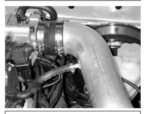
d. Install the upper inlet pipe in the vehicle. Use the reducer coupler and the 2.75" and one of the 3" hose clamps to secure the inlet pipe in place. Install the new breather hose in place and use the hose clamps to secure.
