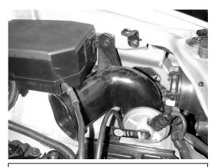
g. Remove the bolt securing the lower inlet pipe and remove from the vehicle.
