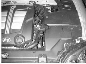
a. Remove the plastic covers covering the stock intake system and battery.
