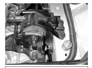
g. Install the rubber soft mount in the threaded hole exposed by the removal of the mounting bracket in step 2(e).
