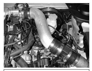
f. Install one of the 3" coupler on the end of the upper inlet pipe and use the supplied 3" hose clamps to secure it to the air flow sensor.
