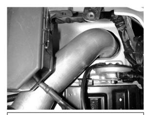
i. The lower intake pipe will pass through the hole in the fender well make sure it is not contacting any part of the body.
