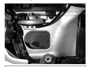
b. The factory hole in which the inlet pipe passes through must be enlarged to make clearance for the AEM CAS Intake pipe.
