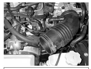
f. Remove the hose clamps securing the stock inlet pipe in place. Remove the breather tube and stock inlet pipe from the vehicle.
