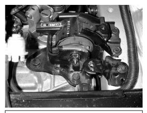
e. Remove the lower filter box support bracket from the vehicle.
