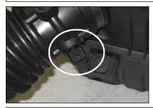
j. Remove the inlet air temperature (IAT) sensor from the stock inlet tube. This may be glued in place so use a sharp knife to cut the glue along the gap and pull the IAT out of the tube.
