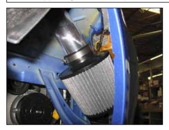
h. Install the air filter on to the end of the lower inlet pipe. Push the filter over the pipe until the stop in the filter is reached. Use a #44 clamp to secure the filter onto the inlet pipe.
