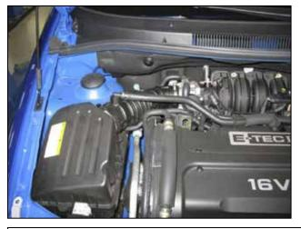
a. Stock air box system installed.
