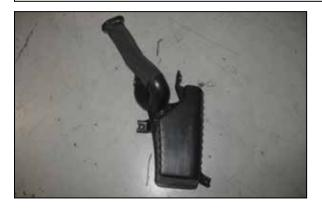
i. Remove the lower intake resonator.
