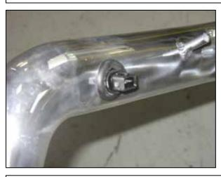
e. Install the supplied grommet into the hole on the inlet pipe. Gently press the IAT sensor into the grommet as shown.
