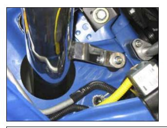
g. Align the inlet pipe mounting bracket with the previously installed rubber mount. Secure the bracket using the supplied M6 washer and nut.
