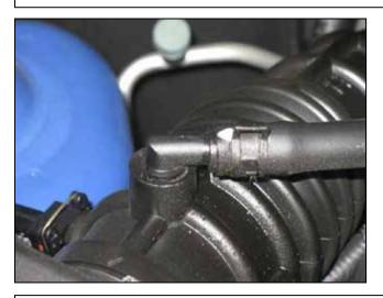
c. Remove the breather hose from the inlet tube.
