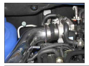
f. Install the inlet pipe into the coupler on the throttle body. This should be done by sliding the bracket side of the pipe through the hole in the inner fender. Secure the pipe using a #40 hose clamp.
