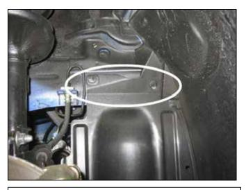
f. From the passenger side wheel well, remove the nut and bolt secruing the inner splash shield to the chassis.
