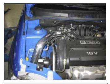
Stock air box system installed.
