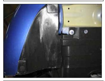
g. From underneath the vehicle remove the two bolts and two plastic connectors holding the splash shields in place. Remove the lower shield and move the fender well liner out of the way.
