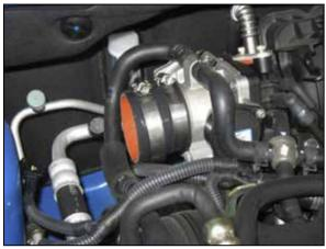
b. Install the straight coupler onto the throttle body and secure using a #40 hose clamp.
