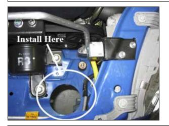
d. Install the supplied rubber edge trim around the hole in the inner fender.
