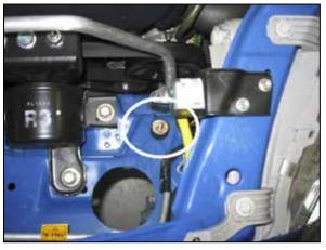
c. Locate the front threaded hole where the stock air filter housing was secured. Thread the supplied rubber mount into the hole in the engine compartment as shown.
