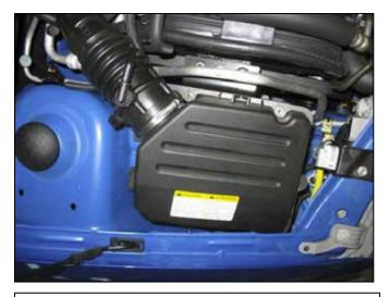
e. Loosen and remove the three bolts securing the air filter housing to the chassis. Remove the housing and the inlet hose by lifting straight up.
