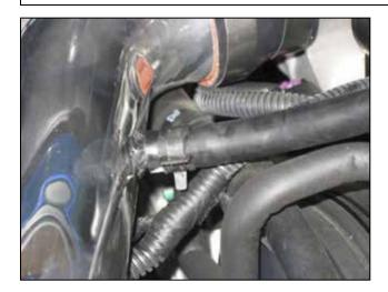
i. Attach the stock breather hose to the nipple on the inlet pipe using the factory spring clamp.
