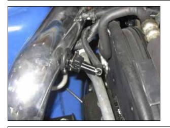
j. Plug the wiring harness into the IAT sensor mounted in the intake pipe. Route the wires under the inlet pipe to avoid scratching the pipe's finish.
