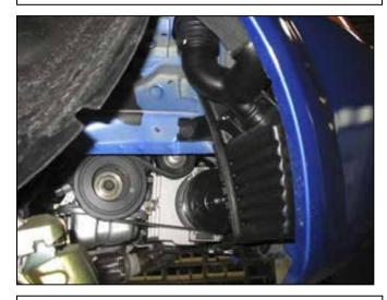
h. Remove the two bolts, one plastic nut, and the plastic retaining clip on the lower resonator and resonator inlet pipe respectively.
