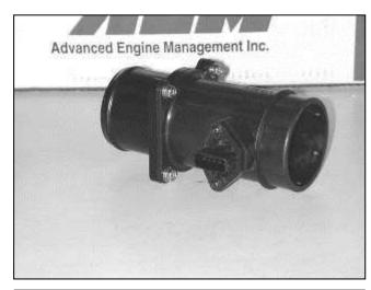
c. Install the included MAF adaptor onto the sensor using the factory bolts as shown.
