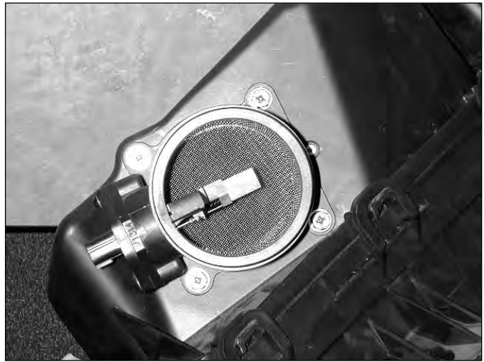
d. Loosen the four bolts, and remove the MAF sensor from the air filter assembly.
