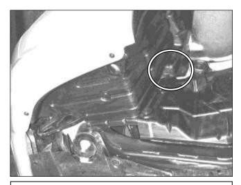
i. Reinstall the inner fender liner. Some trimming of the factory inner plastic may be necessary to clear the rubber mount.
