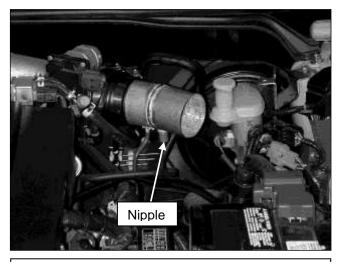
c. Install the upper intake pipe, with the nipple pointing down. Using the supplied coupler and two hose clamps install as shown.
