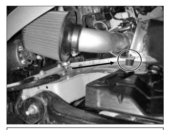
g. Secure the pipe lower pipe to the rubber isolator using the supplied nylock nut and washer.
