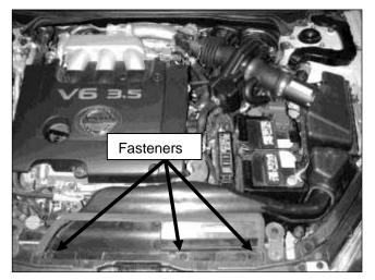
a. Remove the three plastic fasteners that secure the air scoop and remove it.
