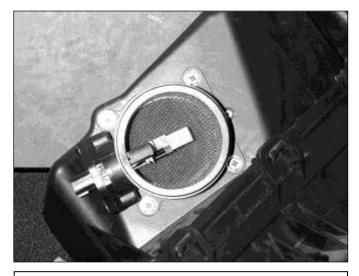
d. Loosen the four bolts, and remove the MAF sensor from the air filter assembly.
