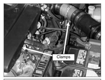
h. Install the included 5/6" breather hose onto the cam cover vent and the nipple on the upper pipe, using the supplied 1" hose clamps.
