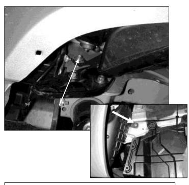
f. Loosen the two indicated bolts, and remove the intake air silencer chamber.
