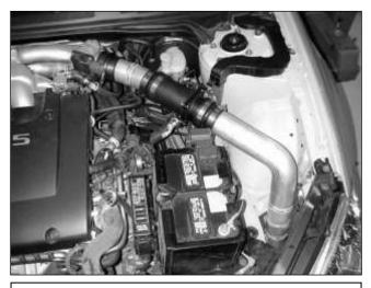
f. Install the lower pipe onto the MAF adaptor, using an included coupler and hose clamps.
