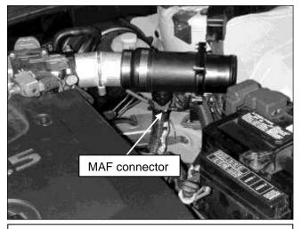
d. Install the MAF sensor on the upper pipe using an included coupler and hose clamps, with the sensor connector facing down, as shown. Reconnect the MAF Sensor.
