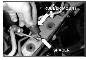
b. Install the rubber mount into the hole that was exposed when the A/C line bracket was removed to step 2j. Use the included spacer underneath the rubber mount to space it upward to clear the bracket. Tighten by hand.
