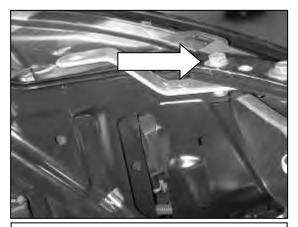
f. Install the 8mm bolt and washer included in the kit into the bolt hole exposed in step 2d. Attach the AEM<sup>®</sup> wiring harness bracket to the bolt on the underside and secure it in place with the included 8mm nylok nut.
