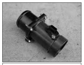
d. Using the four bolts and washers included in the kit, attach the AEM<sup>®</sup> MAF adaptor to the Nissan MAF sensor.
