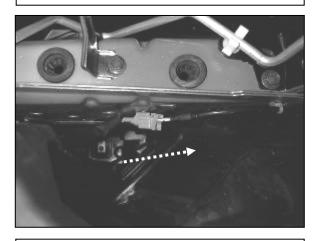
i. Looking where the factory air filter housing was, pull the wheel speed sensor plug shown in the picture from its mount. **NOTE: DO NOT unplug the sensor.**
