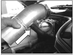
c. Attach the breather hose to the fitting to the AEM<sup>®</sup> upper intake pipe (the shorter one in the kit). Put the 3 ¼" to 3.0" silicone reducer on the end of the pipe closest to the bend. Place the 3 ¼" side of the silicone coupler over the throttle body.
