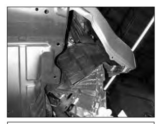
n. It is now possible to gain access to the area behind the front bumper. This is where the air filter will be located.
