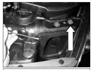
d. Pop out and remove the plastic fastener on the front air duct. Unsnap the duct and slide it forward. Remove the specified bolt as shown.
