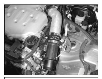
f. Install the assembly from step 3c on the upper intake pipe. Loosely install a #48 hose clamp on the coupler. Make sure the MAF sensor connector is pointing toward the oil cap.
