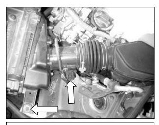
d. Remove the bolt holding the factory air box in place. Unplug the Mass Air Flow (MAF) sensor and unsnap the wiring loom form the intake system.
