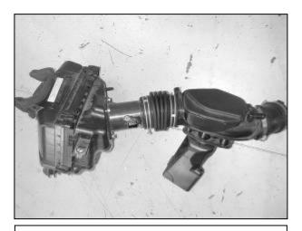
e. Pull directly upward on the air box to unsnap it from the mounts. Remove the complete air box system from the vehicle.
