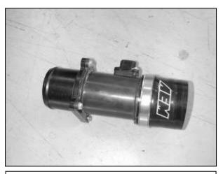
c. Slide one of the 3" straight silicone couplers over the MAF sensor as shown. Lightly oiling the inside of the coupler may help. Secure the coupler in place using a #48 hose clamp.
