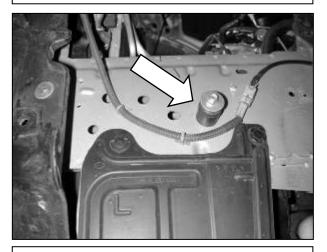
h. Thread the rubber mount into the hole that held the resonant chamber rear mounting bolt. Hand tighten the rubber mount.
