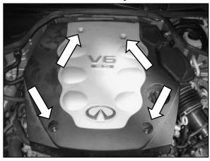
a. Remove the four fasteners holding on the engine cover. Remove the engine cover.
