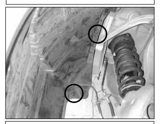
g. From inside the wheel well, remove the two plastic fasteners shown in the picture.
