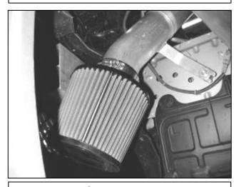
I. Install the AEM® air filter onto the end of the lower intake pipe. Make sure the air filter is fully and squarely seated on the end of the pipe. Use a #52 hose clamp to secure it in place.
