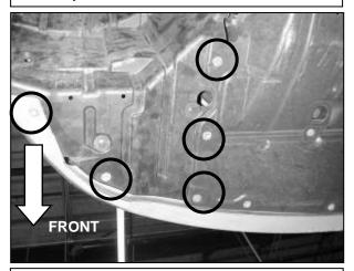
f. From underneath the car, remove the bolts circled in the picture.
