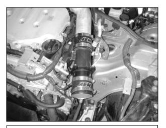
g. Install the other 3" silicone coupler on the end of the AEM $^{\otimes}$  MAF adaptor. Loosely install two #48 hose clamps.
