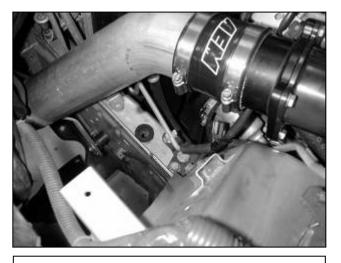
k. Install the lower intake pipe in the end of the coupler on the AEM® MAF adaptor. Line up the bracket on the pipe with the rubber mount and install the 6mm nylock nut and fender washer (See diagram below). Do not completely tighten.
