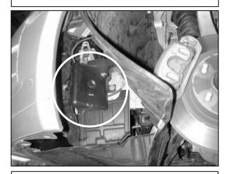
h. Peel back the splash guard and tuck it out of the way. Remove the lower resonant chamber circled in the picture.
