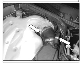
c. Loosen the hose clamp holding the stock intake tube on the throttle body. Loosen the spring hose clamp on the breather hose and pull the hose off of the fitting on the intake tube.
