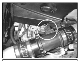
m. Plug in the MAF senor. Place the engine cover on the intake manifold and check for clearance of the MAF sensor plug. Rotate the MAF sensor assembly until the plug has adequate clearance of the cover.
