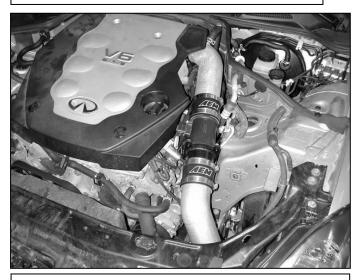
n. Check closely for clearance around the air filter and the AEM® MAF sensor adaptor, reposition as needed.
