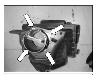
j. Remove the four bolts holding the MAF sensor on the factory air box. Handle the MAF sensor with care.
