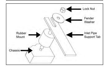
Proper installation of rubber mount assembly.
