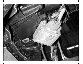
i. If installing on a G35 Sedan, remove the mounting screw for the HID headlight controller.
