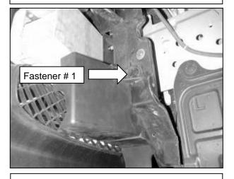
i. Remove the air duct shown by removing the three plastic fasteners holding it in place. (See next page)
