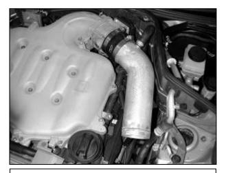
e. Insert the upper intake pipe in the coupler as shown. Reuse the factory hose clamp and install the breather hose on the fitting on the pipe. Do not tighten the #48 hose clamp.
