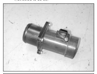
b. Using the 6mm bolts and washers included in the kit, bolt the MAF sensor to the AEM  $^{\!@}$  adaptor.
