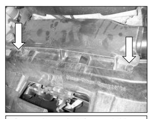
b. Remove the two plastic fasteners holding on the air duct and remove the duct from the engine bay.
