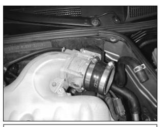
d. Place the 3.25"-3.0" reducing silicone coupler on the throttle body. Use a #52 hose clamp around the throttle body. Make sure the coupler is sitting squarely on the throttle body and tighten the #52 hose clamp. Loosely install a #48 hose clamp on the other end of the coupler.
