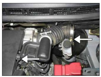
c. Reinstall the factory breather tube and air inlet tube.
