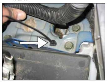
b. Insert the tree mount zip ties into the factory location on the batter bracket. Secure the ECU wire harness to the bracket. Cut off excess tie.
