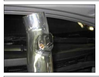
f. Reinstall the MAF Sensor with factory bolts into the AEM $^{\circ}$  inlet pipe.
