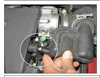
d. Unclasp the spring clamp for the crankcase breather tube. Remove the plastic resonator from the crankcase breather tube.
