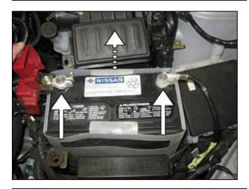
h. Loosen and remove both battery terminals. Remove the battery. With the battery removed, pull the air box out from the mounting grommets.
