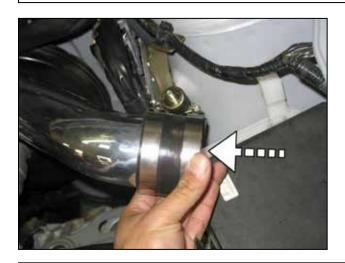
i. Attach the coupler and #40 hose clamps to the installed inlet pipe.
