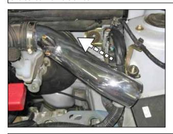
g. Insert the inlet pipe as shown.
