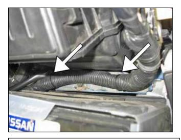
g. Cut the wire tie securing the ECU wire harness to the battery bracket.
