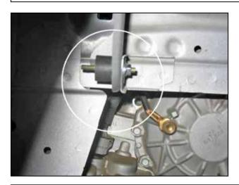
h. Attach the 1" rubber mount in the fender well. Secure the backside of the rubber mount with the M6 washer and M6 Nut.
