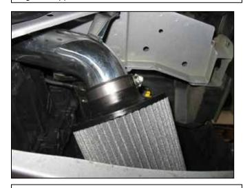
m. Attach the air filter element and secure with #44 hose clamp.
