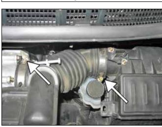
c. Loosen hose clamp at the air box and at the throttle body.
