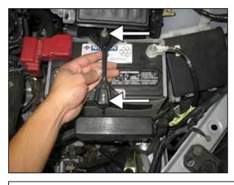
f. Loosen both nuts securing the J-hooks. Remove the J-hooks and battery bracket.
