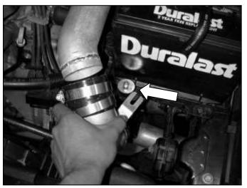
c. Attach the rubber mount to the battery bracket. Attach the lower intake pipe using the provided coupler and hose clamps. Refer to the following diagram for proper installation of the rubber mount.
