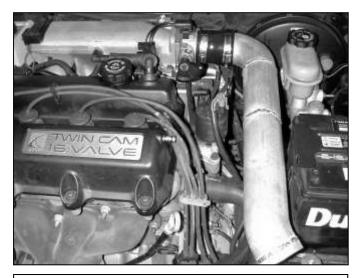
b. Insert the upper inlet pipe with the provided stepped coupler and hose clamps.
