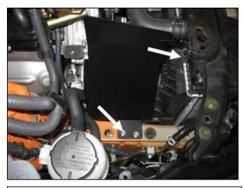
c. **Passenger side**: Insert the heat shield as shown. Secure with new hardware for the base of the heat shield and the factory radiator support bracket.
