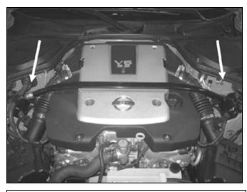
a. Stock intake system. Loosen and remove the bolts and nut on each side of the strut tower bar. Unclip the wire harness from each side. Remove strut tower bar.
