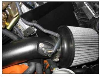
k. Connect the 5/8" hose from the crankcase vents to the intake pipes on both sides (Driver side: 1.75" length, Passenger side: 2" length). Secure with the factory clamp on the plastic nipple and a 1" hose clamp on the pipe side.
