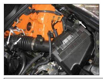
e. Loosen and remove the air box mounting bolt. Loosen the hose clamp at the throttle body. Disconnect the breather hose. Remove inlet tube and air horn mounted in the radiator support.
