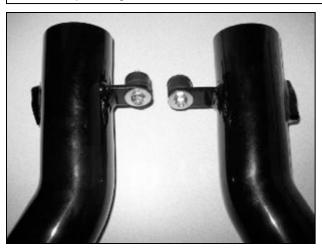
d. Install the rubber mounts on to the brackets on both pipes. Secure with a 6MM fender washer and M6 nut.
