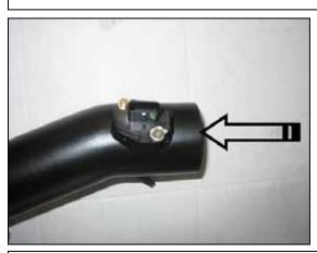
f. Remove the MAF sensors from the factory inlet tubes. Install the MAF sensors into the AEM inlet pipes, use factory hardware.
