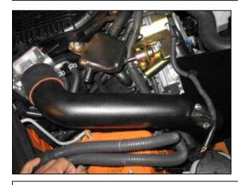
j. Attach the filter and secure with #48 hose clamp. Reconnect the MAF sensor connector.
