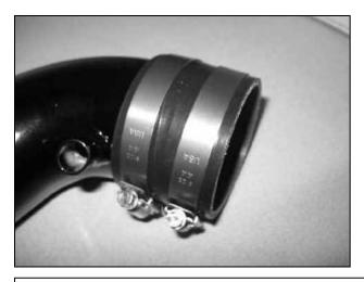
h. Insert the pipe as shown. Align the pipe bracket with the rubber mount. Then align the coupler with the throttle body.
