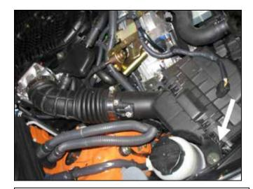
d. Loosen and remove the air box mounting bolt. Loosen the hose clamp at the throttle body. Disconnect the breather hose. Remove inlet tube and air horn mounted in the radiator support.
