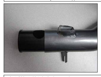
e. Install Venturi into both pipes as shown.
