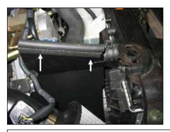
n. Insert the factory MAF wire harness clips into the oval shaped holes on the shields, this applies to both sides.
