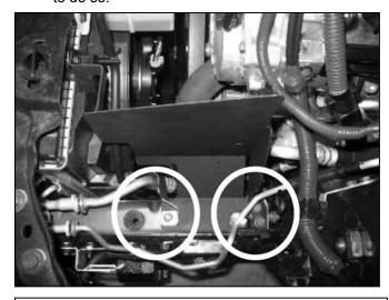
b. Loosen and remove screw that secures the radiator fan to the radiator. This applies to both the driver and passenger side.
