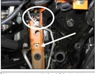
f. Loosen and remove the four A/C line bracket mounting bolts and the rubber grommet that is in between the brackets.
