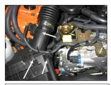
c. Unplug the Mass Air Flow (MAF) Sensor connector and unclip from the air box. Repeat for the driver side.
