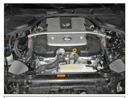
AEM® intake system installed
