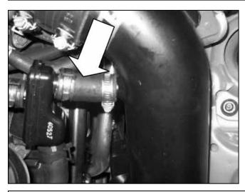
I. Check for clearance. Secure the rubber mount to the shield with a 6MM fender washer and M6 nut.
