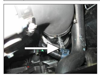
j. Install bracket #32-3058 onto the upper intake pipe's bracket with the supplied bolt #1-2110. Attach the blue harness to the metal clip.
