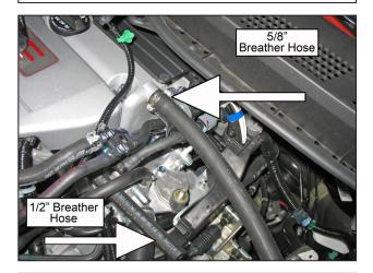
g. Install the two supplied breather hoses, one to the valve cover and the other to the small plastic valve located on the engine. Secure each hose with the supplied hose clamps.
