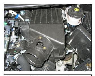
f. Remove the MAF sensor from the air box. Unclip the upper air box from the lower air box.
