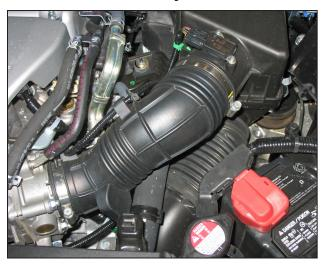
a. Stock air box system installed.
