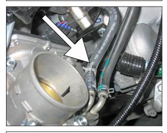
I. Disconnect the coolant line connected to the throttle body.
