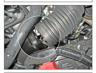
h. Disconnect the lower rubber inlet tube connecting the lower air box to the plastic inlet tube routed through the bottom of the vehicle.
