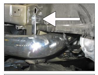
n. Loosely secure the lower intake pipe's bracket to the rubber mount installed in step 3k. Secure the bracket with the supplied washer and serrated nut.
