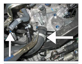
j. NOTE: Ensure the engine is completely cool before removing the coolant hose, or hot coolant will escape from the cooling system and cause injury or damage. To do this, the radiator coolant must first be drained. Follow the procedure described in your vehicle's factory service manual to drain the coolant. Be sure to capture the coolant in an clean container so it can be recycled back into the system in a later step.
