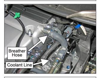
m. Disconnect the breather hose from the valve cover and disconnect the small coolant line connecting the engine to the hard lines.
