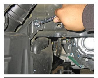
q. Remove the bolt securing the resonator to the inner fender well.
