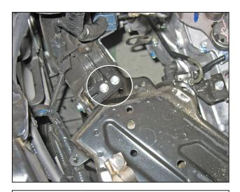
n. Remove the lower inlet tube and the bracket securing the positive battery cable. The bracket securing the positive battery cable has two bolts that will need to be removed.
