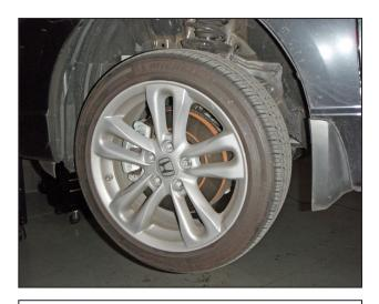
o. Raise the front of the vehicle with a jack. Refer to your owner's manual for proper jack and jack stand placement to properly support vehicle. Support your vehicle using properly rated jack stands before wheel removal or while working under the vehicle. **NEVER WORK UNDER A VEHICLE WITHOUT USING JACK STANDS.** Remove the driver side wheel.
