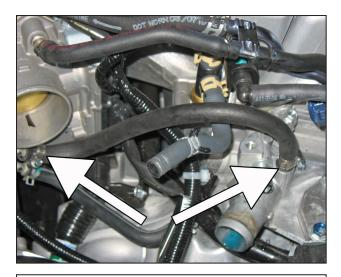
d. Install the supplied 5/16" hose to the throttle body inlet and the engine inlet as shown. Secure each end of the hose with the provided hose clamps.
