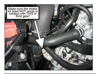
i. Install the intake assembly assembled in step 3c into the elbow. Connect the MAF sensor to the MAF sensor harness connector. Ensure the intake pipe is completely seated into the elbow and is properly positioned so it does not obstruct the shift linkage. Put the vehicle in third gear to ensure that the intake pipe will clear the shift linkage. Connect the two breather hoses installed in step 3g to the upper intake pipe and secure with the supplied hose clamps.
