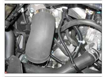
h. Install the elbow coupler onto the throttle body, ensuring it does not contact any of the surrounding parts. Loosely secure it with the supplied #9444 hose clamp.
