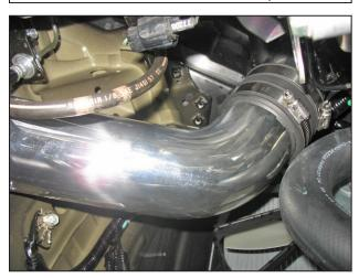
I. Route the lower intake pipe into the engine bay and attach the upper end to the upper intakes pipe's coupler.
