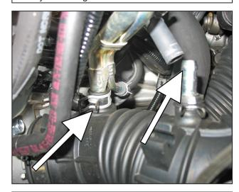
d. Disconnect the two breather hoses connected to the rubber intake tube. One is a hard line and the other is rubber.
