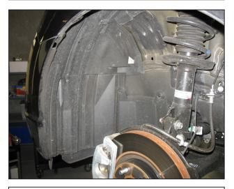
p. Remove the fender liner on the driver side wheel.
