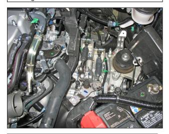
i. Stock air box system removed from the vehicle.
