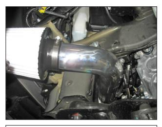
o. Install the air filter onto the lower end of the lower intake pipe. Once proper fitment is achieved secure the air filter to the intake pipe with a #9452 hose clamp.
