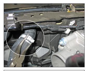
k. Using pliers remove the clamp securing the upper radiator hose to radiator. Remove the upper radiator hose from the vehicle.
