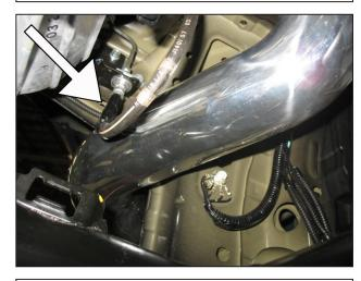
m. Install the supplied helical wrap onto the clutch line where the lower intake pipe passes.
