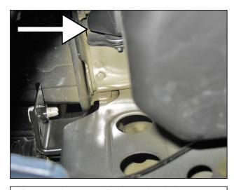
r. Remove the second bolt securing the lower resonator in place; it is located near the front of the vehicle.
