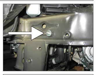
k. Screw the rubber mount into the threaded hole of vehicle's frame.
