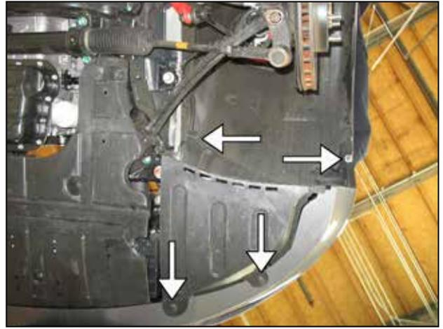
f. Lift the car and remove the right front wheel. From underneath the vehicle, remove three clips and one screw from the inner wheel well liner. Pull the wheel well liner back out of the way.
