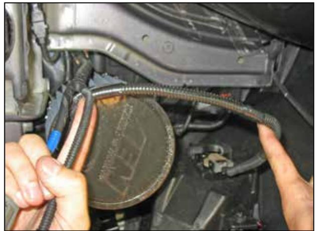
o. Install the supplied section of wire loom on the exposed fog light wires and secure it with tape. Unclip the washer fluid hose from the clip that attaches it to the inner fender, and push the hose and two wire connectors up top behind the headlight.
