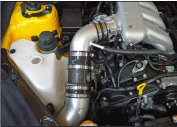
l. Install the lower pipe with the 4.0" x 2" coupler and two #64 clamps. Align the bracket with the rubber mount and secure it with the washer and M6 nut.
