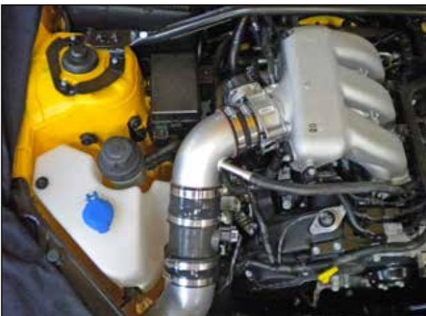
p. Plug in the washer pump and washer fluid level sensor. Reattach the washer fluid hose to the pump and fill up the washer bottle, then snap on the blue washer fluid cap.
