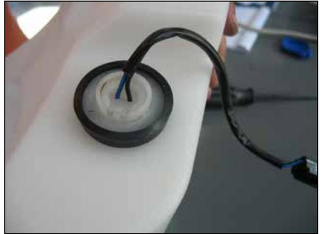
e. Apply liquid soap solution to the level sensor and insert it into the grommet. Make sure that the level sensor is pressed all the way into the grommet. The lip of the sensor should be inside the groove of the grommet.
