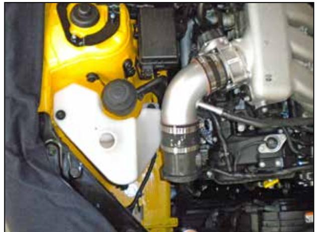
k. Install the washer bottle assembly and attach it with two of the M6 bolts removed in step 2d.
