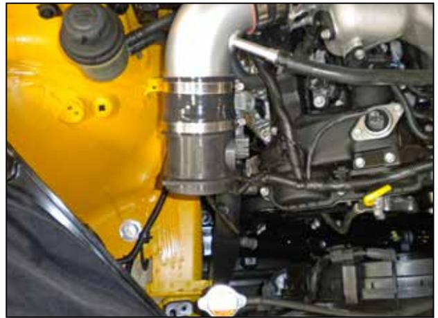
i. Attach the MAF sensor to the upper pipe as shown using the 3.5" x 3" coupler and two #60 clamps. Be sure that the MAF sensor is oriented as shown, and arrow on the MAF is pointing toward the engine.
