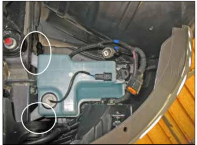
h. Remove two M6 bolts securing the washer bottle. Unplug the hose from the washer pump and remove the washer bottle from the car. Drain any remaining washer fluid into a clean container so it can be reused.
