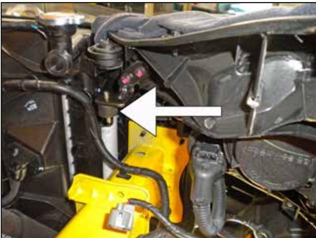
j. Install the supplied M6 rubber mount from the underside of the bracket as shown.
