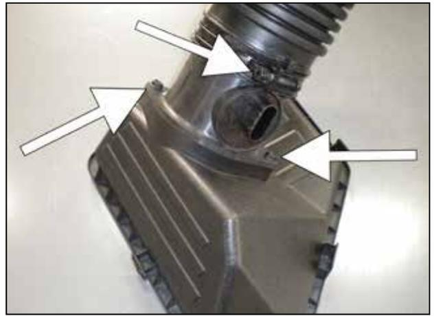
g. Disassemble the MAF from the airbox by removing the two screws. Also loosen the clamp securing the rubber inlet hose to the MAF and remove the hose.
