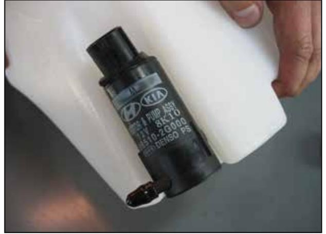
c. Apply some liquid soap solution to the washer pump and insert it into the grommet. Firmly press the pump all the way into the grommet.
