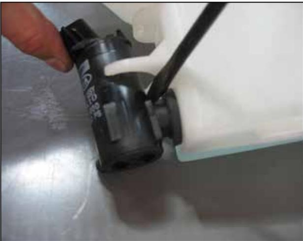
k. Pry the washer pump out of the grommet and set it aside. Also remove the grommet and set it aside.
