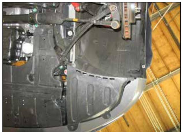
q. Reinstall the fender liner and wheel.
