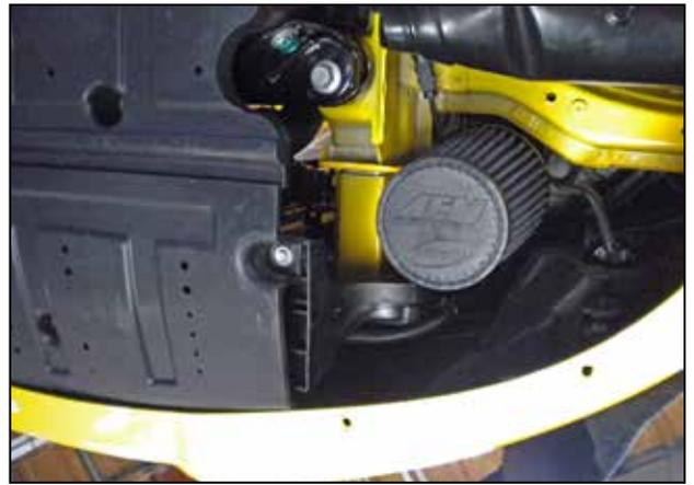
m. From underneath the car, install the filter with the #64 clamp. Slide the filter onto the end of the pipe until the pipe reaches the stop inside the filter, then tighten the clamp.
