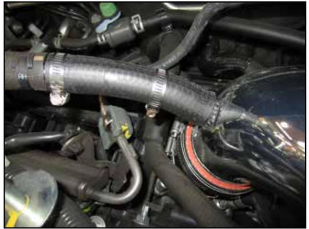
m. Install the (7) hose onto the (1) intake tube and insert the (8) nipple into the OEM vent hose as shown.
