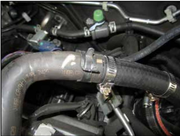
n. Secure the vent hose on the nipple with the OEM clamp.
