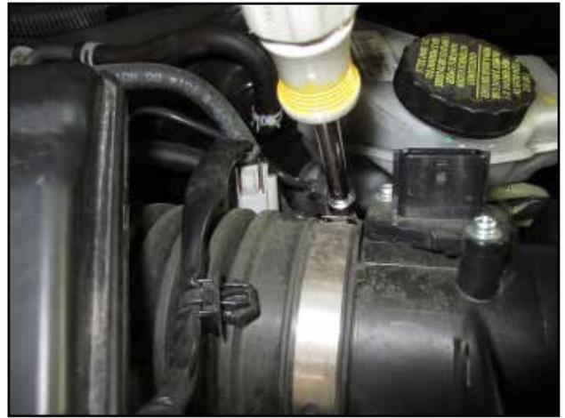
f. Loosen the hose clamp on inlet tube to the airbox.
