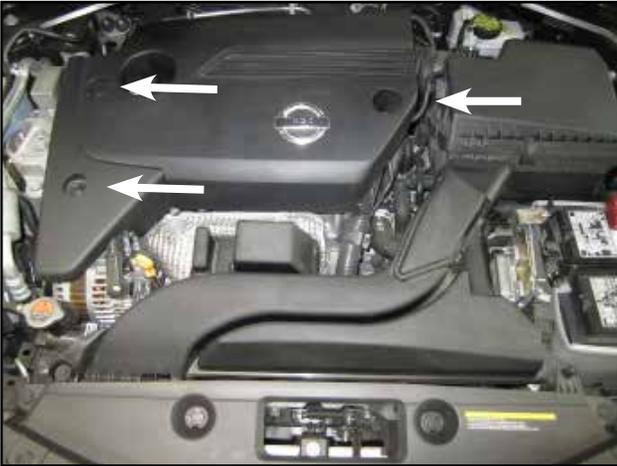
a. Remove the three Allen head bolts that secure the engine cover in place.
