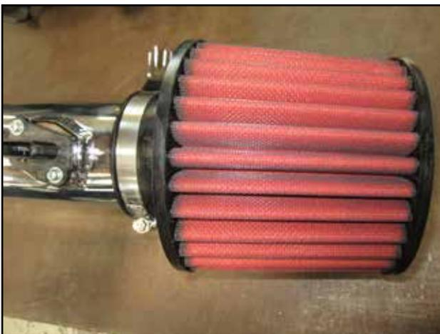
j. Mount the AEM air filter (2) onto the intake tube (1) using the (6) hose clamp. Tighten Hose clamp.
