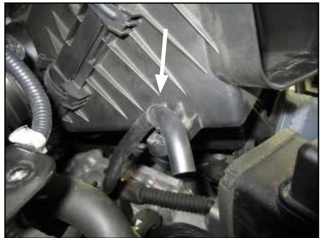
h. Undo the clip on the airbox holding the transmission vent hose. Undo the transmission vent hose clip from the airbox.
