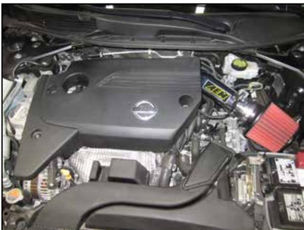
r. Make sure all the hose clamps and fasteners are tight then install the engine cover.
