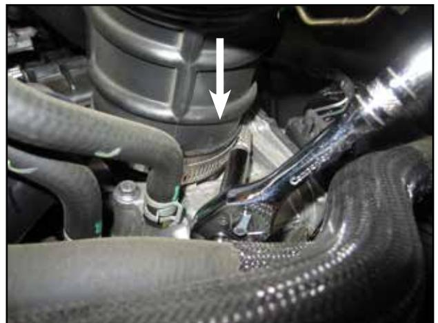
j. Loosen the hose clamp on inlet tube to the throttle body and remove hose.
