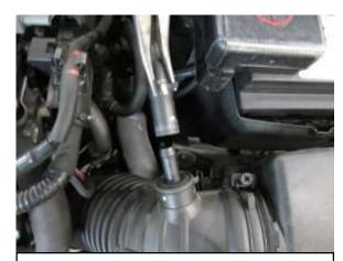
B. Disconnect the breather return hose at the stock intake tube.
