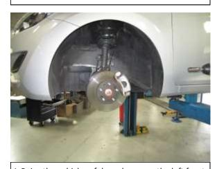
J. Raise the vehicle safely and remove the left front (driver's side) wheel. Make sure to set the parking brake, chock the rear wheels, and use proper jack stands before working under the vehicle.
