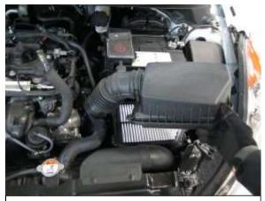
E. Unfasten the air box clamps and remove the stock air box lid and intake tube.
