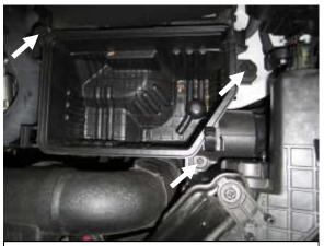
G. Remove the three M6 mounting bolts with a 10mm socket. Slide the lower air box housing to the left and remove it from the engine bay.
