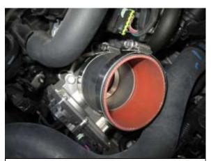
A. Install two #48 hose clamps (F) onto the silicone hose (E), then install the hose over the throttle body flange. Tighten the hose clamp over the throttle body flange and leave the other clamp loose.
