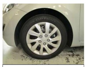
K. Re-install the driver's side wheel and torque down the lug nuts to the factory specifications found in your Vehicle Owner's Manual using a torque wrench.
