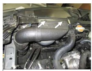
H. Depress the center buttons of the two plastic clips retaining the stock intake scoop to the radiator support. Pull up on the clips to remove them, then remove the stock intake scoop.
