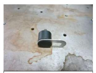
C. On 2014 up models assemble the supplied adapter bracket, rubber mount and rubber insulator pad as shown. 2014 up models require the use of this adapter due to location change of the threaded hole.
