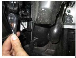
L. Inside the wheel well area, remove the three M6 bolts retaining the intake silencer to the frame support.
