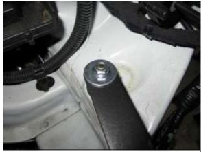
E. Loosely install the flat washer (C) and M6 flanged hex nut (D) over the M6 mounting stud as shown. Do not tighten yet.
