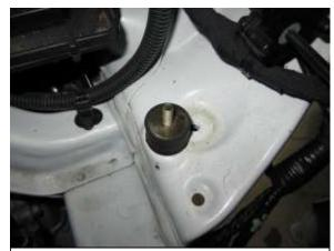
B. On 2011 to 2013 models Install the insulated M6 mounting stud (B) into the fender well and fully tighten by hand. Use the M6 threaded hole to the left of the hole actually used to mount the stock air box.
