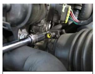
D. Loosen the hose clamp at the throttle body.
