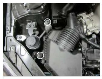
f. Remove the two bolts shown that secure the stock air box to the vehicle. Then remove the air box. **NOTE:** Do not discard any of your stock intake equipment.
