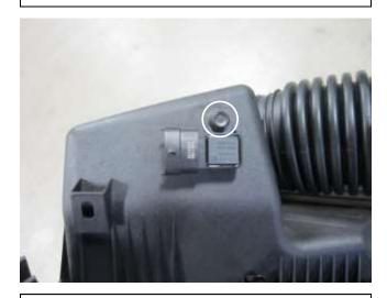
j. Loosen the bolt that secures the temperature sensor to the air box. **Note:** These will be reused in step 3a.
