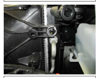
h. Remove the bolt on the front fan shroud. **Note:** These will be reused in step 3d.
