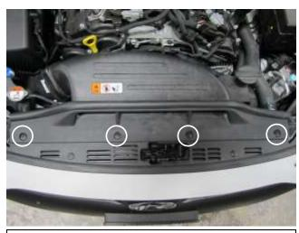
b. Remove the 4 plastic screws that hold down the air scoop. Note: These will be reinstalled in step 3p.
