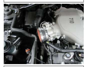
h. Install the coupler (5-351)and hose clamps (9456) onto the throttle body. Tighten the hose clamp on the throttle body side at this time.
