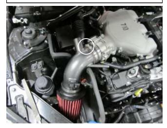
j. Install the AEM intake tube into the coupler and tighten the other hose clamp.
