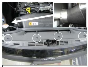
p. Install the scoop into the vehicle aligning the scoop adapter into the hole in the heat shield. Reinstall the engine cover.
