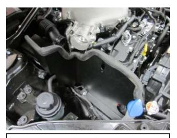
f. Install the edge trim (102496) onto the heat shield at this time.
