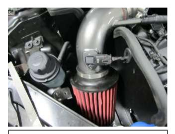
m. Connect the temperature sensor connector to the sensor.
