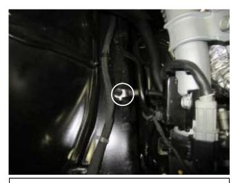
g. Remove the ground strap bolt located underneath the air box. This bolt will not be reused.
