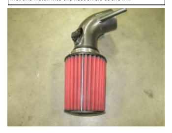
i. Install hose clamp (9456) and AEM filter onto the intake tube. Tighten clamp.
