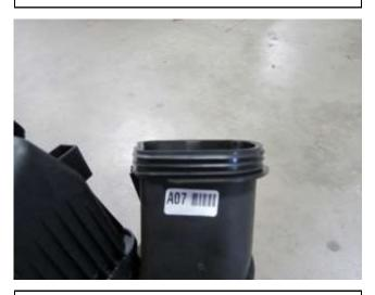
i. Remove the seal off of the stock air box. **Note:** This will be reused in step 3n.
