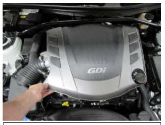
a. Pull up on the engine cover and remove it.
