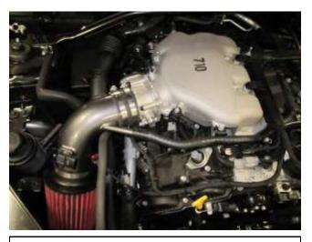
I. Slide the vent tube onto the AEM intake and secure with the stock spring clamp.
