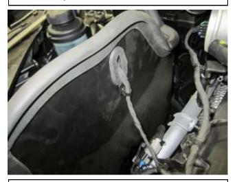
g. Slide the temp. sensor connector through the grommet (784640) and heat shield, then squeeze the grommet and install into the heat shield as shown.
