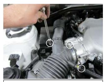
e. Loosen the hose clamps at the sound tube, the throttle body, and unclip the spring clamp on the vent line.
