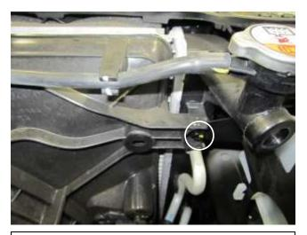
d. Align the heat shield flange with the fan shroud and install the bolt that was removed in step 2h.
