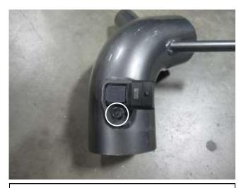
a. Install the temperature sensor into the AEM intake tube and secure with the bolt removed in step 2j.
