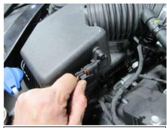
c. Unplug the intake temperature sensor by depressing the clip and pulling away from sensor.
