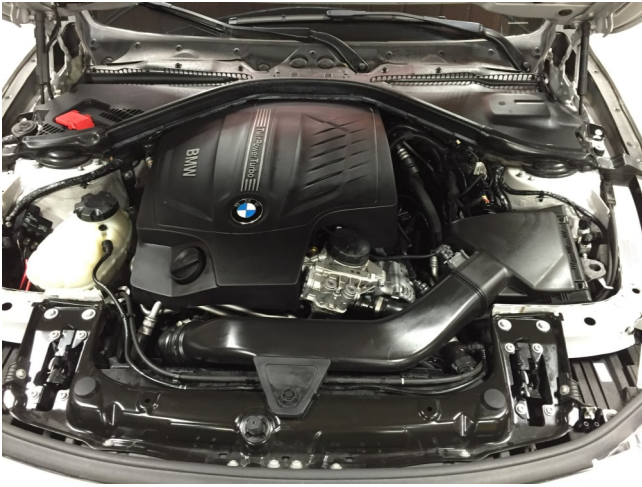
STOCK INTAKE INSTALLED
