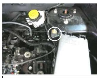
f. Install the rubber mounted stud onto the inner fender as shown.
