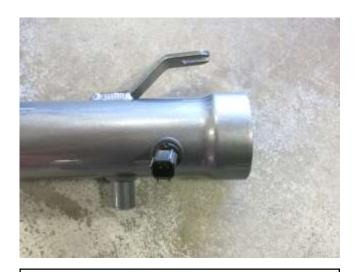
c. Install the air temperature sensor that was removed in step 2i. into the grommet.
