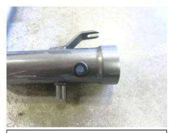
b. Install the provided grommet into the hole on the AEM intake tube.
