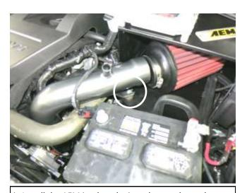
j. Install the AEM intake tube into the coupler at the throttle body and align the bracket with the rubber mount.
