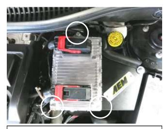
h. Place the ECU onto the heat shield and install the three bolts that were removed in step 2c. Note: Make sure to connect the ground strap.
