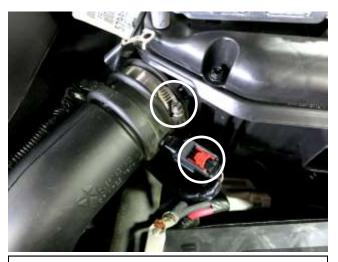
b. Slide the red locking tab and disconnect the intake air temperature (IAT) sensor from the stock intake. Loosen the hose clamp circled.
