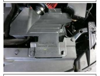
p. Install the fresh air scoop back onto the vehicle that was removed in step 2a.
