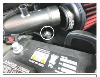
I. Install the provided hardware and secure the AEM intake tube to the rubber mount.
