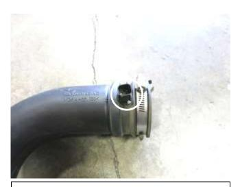
i. Remove the air temperature sensor from the stock intake tube. This will be reused in step 3c.
