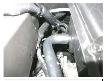
e. Remove the vent hose on the side of the stock air box. This will be reattached in step 3o.
