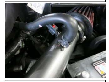
o. Install the vent tube that was removed in step 2e. onto the AEM intake tube with the provided spring clamp.
