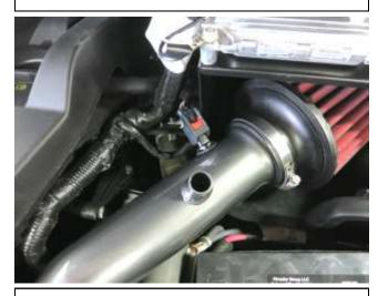
n. Plug the air temperature sensor connector into the air temperature sensor and lock the red locking tab.
