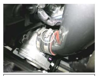
k. With the AEM intake tube aligned in the hose, tighten the hose clamp circled.
