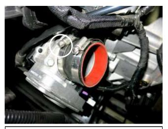
a. Install the provided hose and hose clamps onto the throttle body. Tighten the hose clamp closest to the throttle body at this time.
