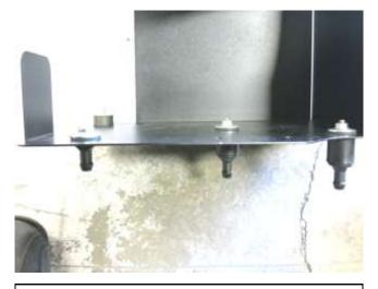
d. Install the provided hardware onto the AEM heat shield. Refer to the exploded view for hardware orientation.
