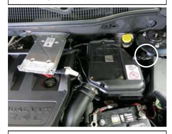
d. Carefully lay the ECU over the engine cover and remove the bolt securing the air box mounting bracket to the inner fender.
