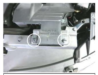
a. Twist the two plastic clips that secure the fresh air scoop to the vehicle and remove the scoop. This will be re-installed in step 3p.
