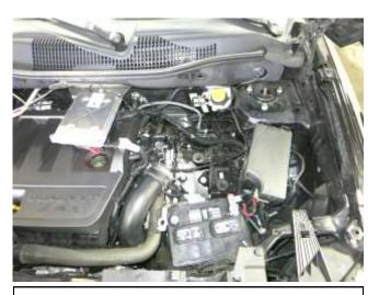
g. Remove the stock air box from the vehicle. Note: Do not discard any of your stock equipment.
