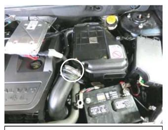
f. Disconnect the stock intake tube from the stock air box.
