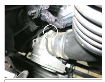
h. Loosen the hose clamp securing the stock intake tube to the throttle body and then remove the intake tube from the vehicle.
