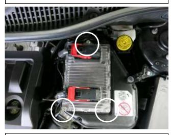
c. Remove the three bolts securing the ECU and ECU ground to the air box lid. Then flip the ECU over and lay it on the engine cover. NOTE: It is NOT necessary to disconnect the ECU electrical connection. The bolts will be reused in step 3h.
