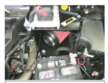
i. Place the AEM air filter with the hose clamp into the heat shield at this time.
