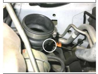
h. Install the hump hose onto the turbo compressor and tighten the clamp closest to the turbo at this time.
