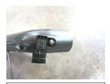
c. Install the electrical sensor that was removed in step 2j. into the AEM intake tube and secure with the provided hardware.
