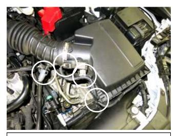
b. Disconnect the electrical connector, the two wiring harness connectors, and the vent tube on the stock intake.
