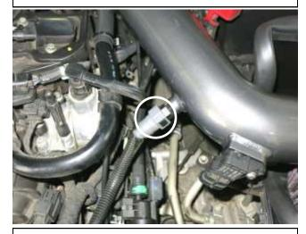
n. Reconnect the vent line onto the AEM intake tube that was removed in step 2b.
