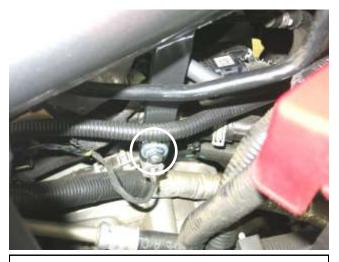
I. Once proper alignment is achieved, install and tighten the provided washer and nut onto the rubber bushing that was previously installed in step 3d.
