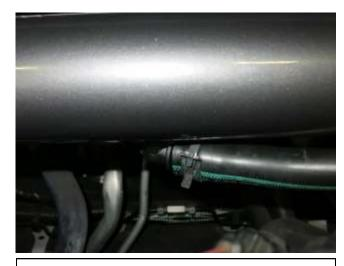
q. Slide the vent tube over the 90° fitting and secure with the spring clamp.
