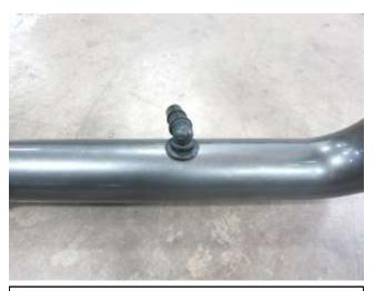
b. Install the provided grommet and 90° vent fitting into the AEM intake tube.
