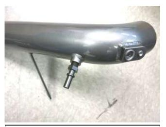
a. Install the provided vent fitting into the AEM intake tube as shown.
