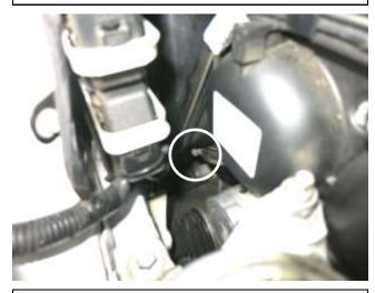
h. Loosen the hose clamp at the turbo compressor and remove the stock intake tube from the vehicle. Note: Do not discard any of your stock equipment.
