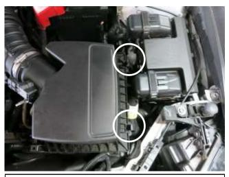
c. Unlatch the two clips that secure the upper to the lower air box.
