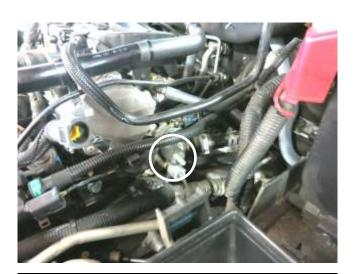
d. Install the rubber mounted stud onto the engine as shown.
