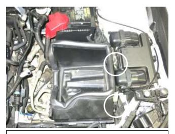
f. Place the assembled heat shield into the vehicles lower air box and secure with the clips that were unlatched in step 2c.
