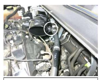
f. Squeeze to release the vent connector from the stock intake tube that leads to the turbo.
