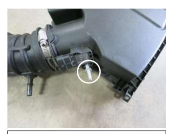
j. Using a E5 TORX socket remove the bolt securing the electrical sensor to the upper air box. This will be reused in step 3c.
