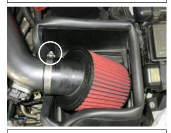
p. Attach the filter to the AEM intake tube and secure it with the hose clamp.
