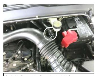
d. Unclip the vent line from the stock intake.
