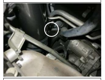
m. Once proper alignment is achieved, tighten the hose clamp securing the AEM intake tube to the hump hose that was previously installed in step 3h.
