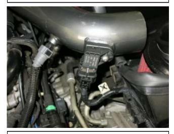
o. Install the electrical connector back onto the sensor that was removed in step 2b.
