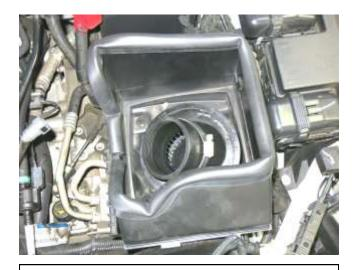
j. With the hose clamp on the filter loosely, lower the filter into the lower air box as shown.
