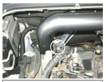
r. Install the engine cover stand that was removed in step 2g. and re-install the vehicle engine cover.
