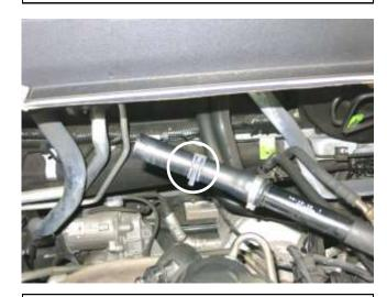
i. Install the provided spring clamp onto the vent line as shown.
