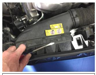
b. Release factory inlet duct with a small flat blade as shown and pull downward to fully disconnect.
