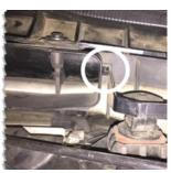
h. Release the inlet cover by squeezing and pushing the cover retainer tabs located on either side of the secondary inlet.
