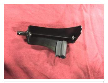
f. Install the 40mm trim piece on the airbox stand-off and assemble remaining components onto it as shown above.
