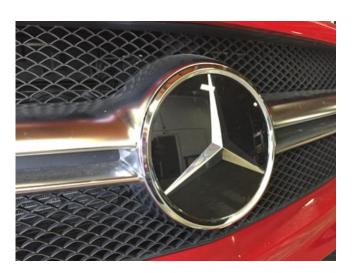
g. To open up maximum airflow to intake, the secondary air inlet must be uncovered. Twist the Mercedes emblem on the grill counterclockwise and pull to remove it. If your car is equipped with Distronic radar-assisted parking and cruise control features, this emblem (shown at right above) will not be removable by twisting in this fashion. The grill will need to be removed to allow removal of the cover as detailed in step 3h below.
