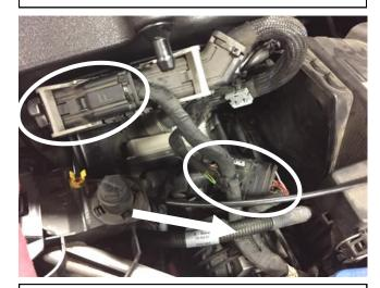
h. Disconnect the two wiring harnesses circled above and pass them under the conduit indicated by the arrow above. Reconnect them both before proceeding.
