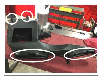
a. Install the airbox mounts on the airbox and trim the supplied edge trim to fit the front air inlets in the airbox.
