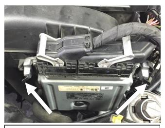
d. Disconnect the ECU mount clips by pushing on them in the direction indicated by the arrows above, then lift the ECU away from the airbox and set aside.
