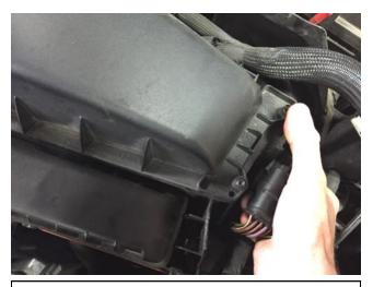
e. Lift up on wire harness retainer on the side of the airbox to remove it.
