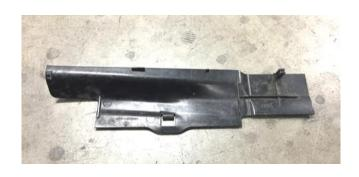
i. The inlet cover may now be removed through the emblem hole. It will look like the piece above. Replace the emblem at this time. Installation is reverse of removal.
