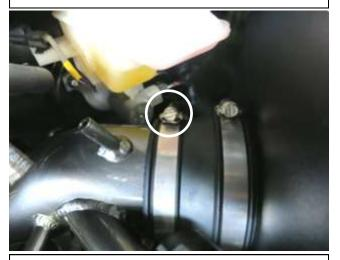
n. Tighten the hose clamp on the coupler at the heat shield.
