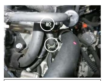
j. Follow the hard line from the previous step to the "T" fitting. Remove the short vent line and spring clamps from the hard line to the "T" fitting. The spring clamps will be reused in step 3g & 3i.
