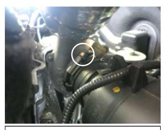
f. Loosen the hose clamp at the turbo compressor.
