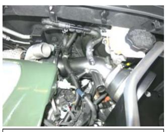
I. Push the heat shield down to secure the stand-off into the grommet in the vehicle while aligning the intake tube with the coupler.
