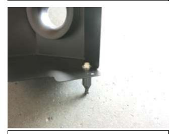
d. Install the stand-off and provided hardware onto the heat shield. You will install it on the inside hole.
