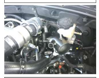
j. Install the AEM intake tube into the coupler at the turbo compressor. Note: Soapy water will help installation and adjustment.
