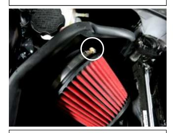
p. Install the AEM filter onto the filter adaptor and tighten the hose clamp.
