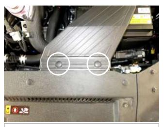
r. Install the stock scoop back into the vehicle with the clips that were removed in step 2a.
