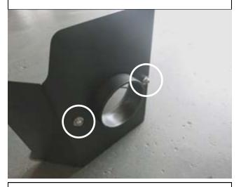
c. Install the filter adaptor with the provided hardware onto the heat shield as shown.
