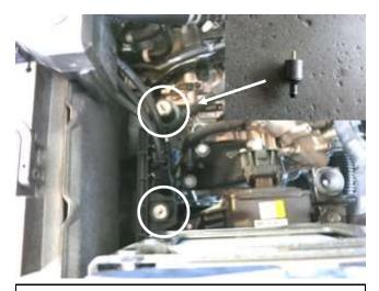
a. Install the provided rubber bushings and plastic mount into the vehicle. Note: You will screw one bushing into the plastic mount as shown in corner of picture.
