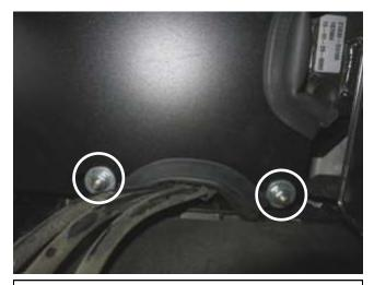
k. Install the completed heat shield into the vehicle aligning the slots in the shield to the previously installed studs. Install the washers/nuts and tighten.
