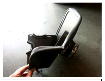
f. Install the provided edge trim onto the completed heat shield. Note: Some trimming may be necessary.
