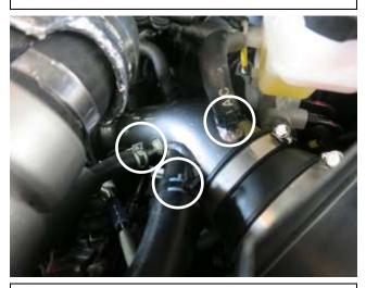
o. Install the vent hoses and spring clamps that were removed in step 2c.
