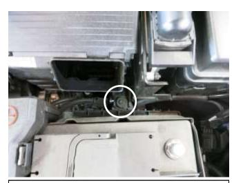
d. Remove the bolt behind the battery that secures the stock air box to the engine compartment.
