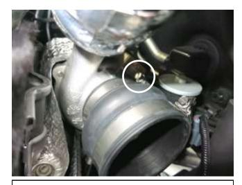
b. Install the provided coupler and hose clamps onto the turbo compressor inlet. Tighten the hose clamp circled at this time.
