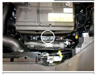
b. Remove the battery hold down bolt and bracket. Then slide the battery as far forward as possible. The bolt and bracket will be reinstalled in step 3g.
