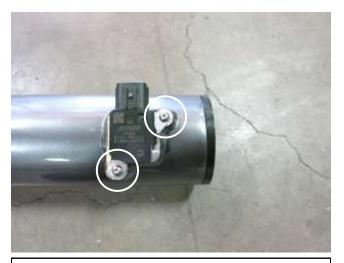
b. Install the MAF sensor into the AEM intake tube and secure with the provided hardware.
