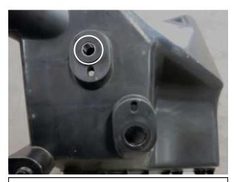
n. Turn the lower air box over and remove one of the metal sleeves and rubber grommet. The metal sleeve will be reused in step 3E.
