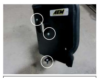
f. Assemble the adapter and air box mount with the provided hardware according to diagram on pg. 2.
