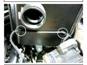
i. Secure the MAF sensor wiring harness onto the AEM heat shield via the stock clips. Then, lower the heat shield into the engine bay and press the air box mount into the stock grommet.
