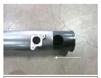
a. Install the venturi into the AEM intake tube, be sure the two openings are aligned.
