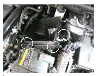
I. Maneuver the lower air box to access the three pushin wire harness clips and disconnect all of them.
