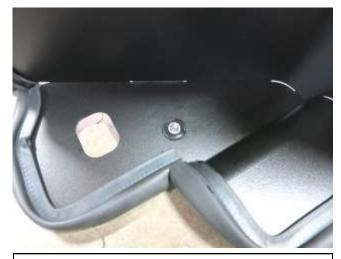
e. Take the sleeve that was removed in step 2n and install it into the grommet. **Note: A little soapy water will ease installation.**
