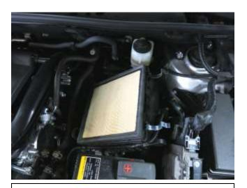
j. Remove the stock air filter from the lower air box.
