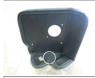
d. Install the edge trim as shown around the AEM heat shield, trim off excess if necessary. Then, install the provided grommet into the hole shown.
