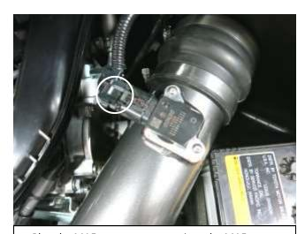
n. Plug the MAF sensor connecter into the MAF sensor.
