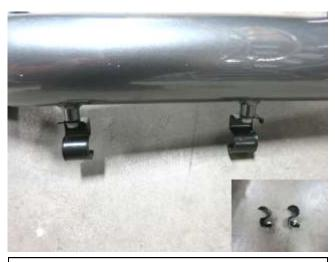
c. Take the stand-offs and bolts from step 2p. and install the bolts according to the inset picture. Then, install them onto the AEM intake tube as shown.
