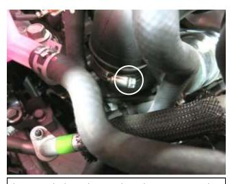
d. Loosen the hose clamp at the turbo compressor inlet.
