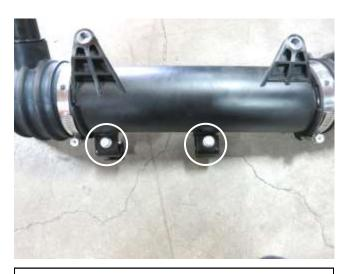
p. Remove the two bolts and stand offs. These will be reused in step 3c.
