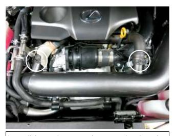
I. Install the vent hoses onto the AEM intake tube and secure with the spring clamps removed in step 2b.
