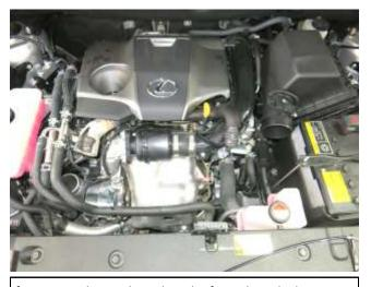
f. Remove the stock intake tube from the vehicle.
