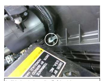
h. Slide the wire loom clip off of the air box.
