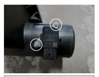
o. Remove the two screws that secure the MAF sensor to the upper air box. The MAF sensor will be reused in step 3b.
