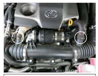
b. Squeeze to loosen the spring clamps and disconnect the vent hoses from the stock intake tube.
