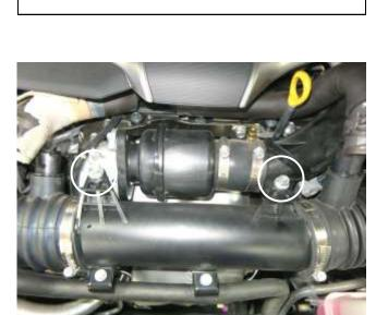
c. Loosen and remove the two bolts securing the stock intake tube to the vehicle.
