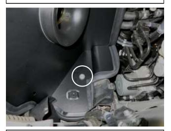
j. Align the grommet/sleeve with the mounting hole in the vehicle and use the factory bolt removed in step 2k to secure the heat shield to the vehicle.
