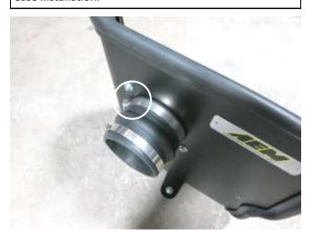
g. Install the hump hose onto the adapter with the provided hose clamps. Tighten the hose clamp closest to the heat shield at this time.
