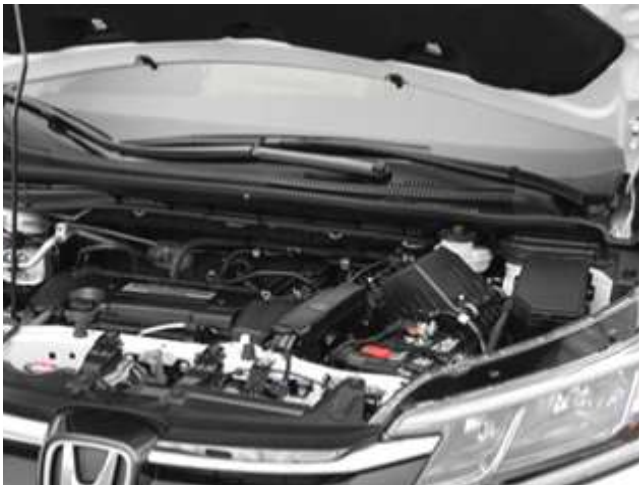
STOCK AIR BOX INSTALLED
