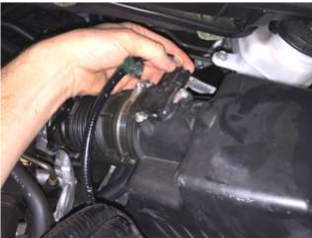
c. Disconnect the mass airflow sensor (MAS) wiring harness and disconnect the wiring retainer clip from the air box. Remove the sensor from the air box and set aside along with its screws to be reused in step 3f.
