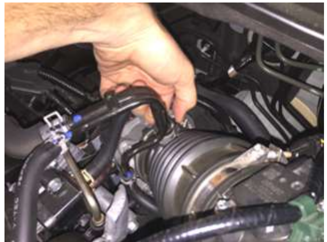
d. Disengage the spring clamp as shown and pull out the steel PCV line from the top of the factory coupler.
