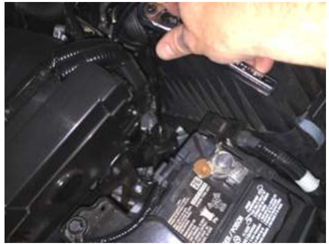
b. Remove the lower bolt securing the factory air box.
