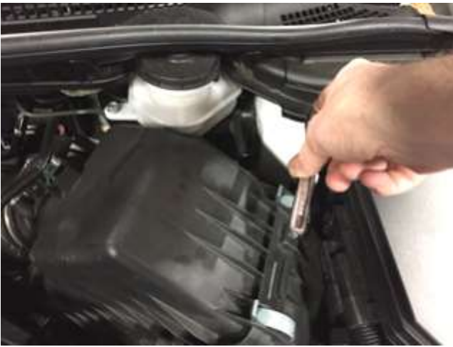
a. Remove the upper bolt securing the factory air box.
