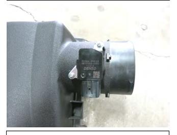
j. Use a small Phillips head screwdriver to unfasten the 2 Phillips head screws and remove the MAF sensor from the upper air box. Do not discard any of the stock equipment removed thus far.
