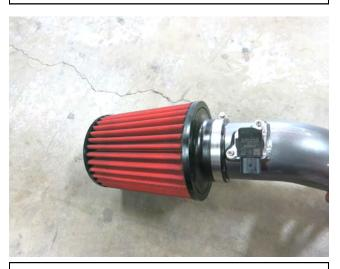
c. Attach the air filter, with the large hose clamp, to the intake pipe. Use an 8mm socket and ratchet, or a flat head screw driver, to tighten the hose clamp to 30 in-lbs.
