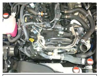
f. Loosen the hose clamp holding the intake tube onto the turbo inlet pipe. Then, remove the intake tube.
