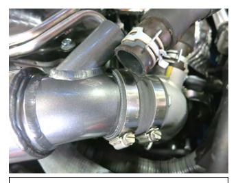
I. Tighten the hose clamp, holding the intake pipe to the coupler, to 30 in-lbs.
