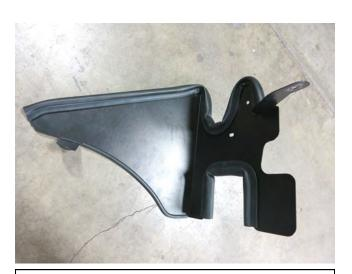
d. Apply the supplied edge trim to the heat shield, as shown above.
