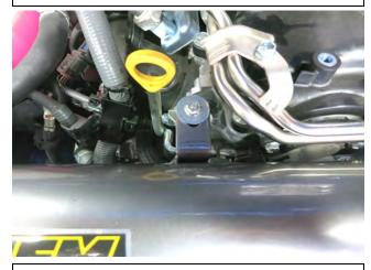
j. Adjust the intake pipe for best fitment, making sure it isn't hitting any surrounding components. Then, fasten the mounting bracket to the soft mount with the supplied fender washer and M6 flanged nut.
