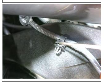
o. If there is too much tension on the MAF sensor harness, you can adjust the position of the wire ties. Use a small flat head screwdriver to relieve tension on the wire tie. Then, you can slide the wire tie along the harness as necessary.
