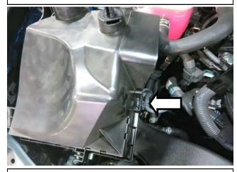
i. Flip the lower air box around. Remove the wire tie from the air box. Remove air box from vehicle.
