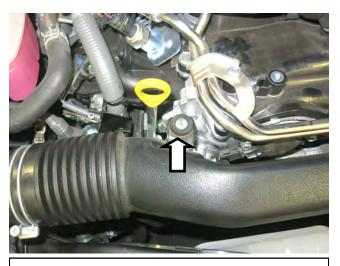
d. Remove the M6 bolt holding the intake tube to the engine.
