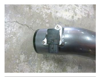
b. Attach the MAF sensor to the intake pipe using the 2 provided M4 bolts.
