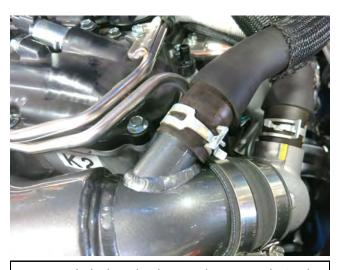
m. Reattach the breather hose to the port on the intake pipe.
