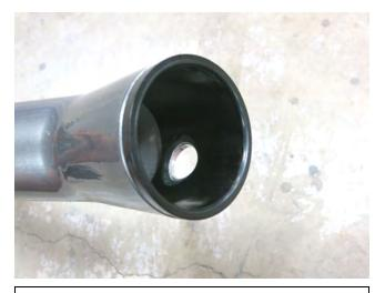
a. Insert the venturi into the AEM intake pipe. Make sure the cutout in the venturi aligns with the cutout in the intake pipe.
