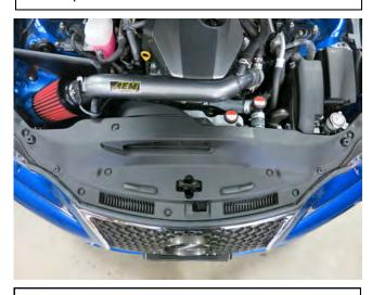
q. Replace the radiator shroud with the 9 push clips you removed in step 2a.
