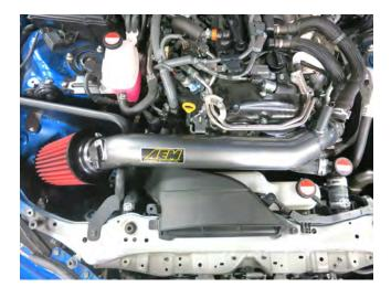
i. Insert the assembled AEM intake pipe into the turbo inlet pipe coupler. Make sure the mounting bracket on the intake pipe aligns with the soft mount.
