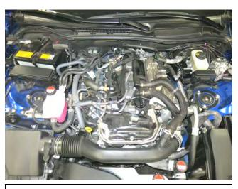
b. Carefully pull up on the engine cover and remove it.
