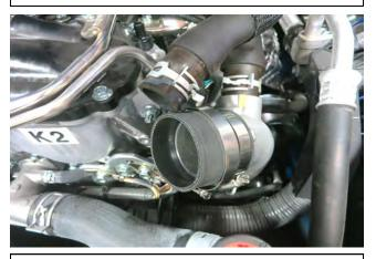
h. Place the tapered, reinforced coupler onto the turbo inlet pipe. Make sure the smaller diameter end is on the turbo inlet side. Then, place the 2 small hose clamps onto the coupler. Leave the hose clamp on the intake pipe side loose. Tighten the hose clamp on the turbo inlet side to 30 in-lbs.
