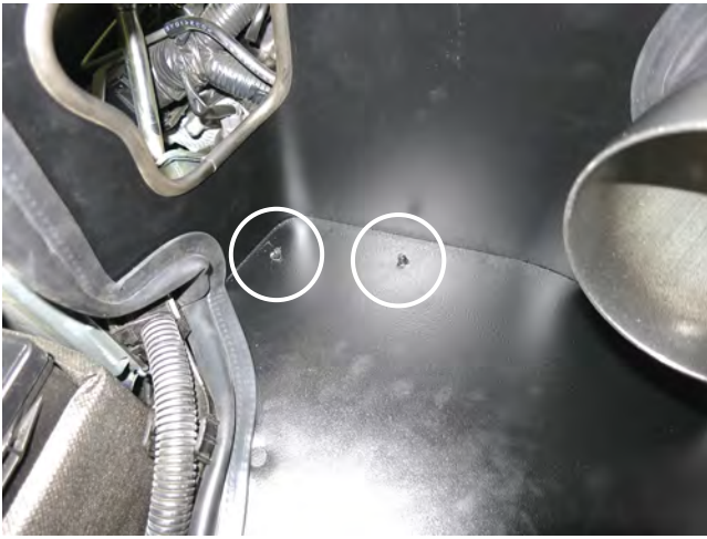
i. Install the transmission vent line clips to the heat shield from the bottom.
