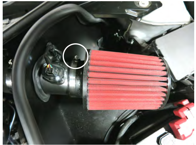
l. Install the AEM filter onto the AEM intake tube and tighten the hose clamp to 30 in. lbs.
