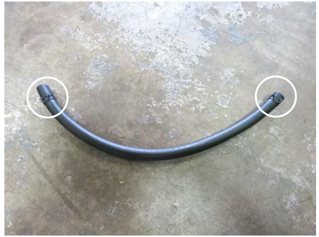
j. Install the spring clamps that were removed in step 2c. onto the provided vent line as shown.
