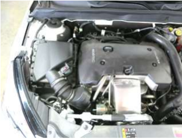
STOCK INTAKE INSTALLED
