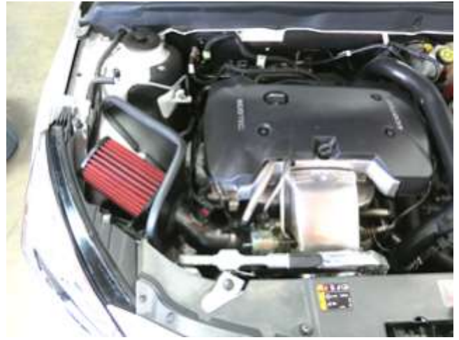
AEM INTAKE INSTALLED
