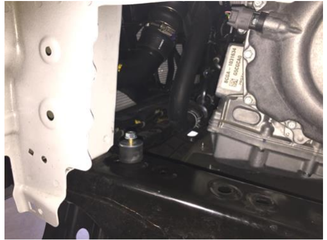
a. Install the provided rubber mount, nut and washer where the resonator support bracket was removed.
