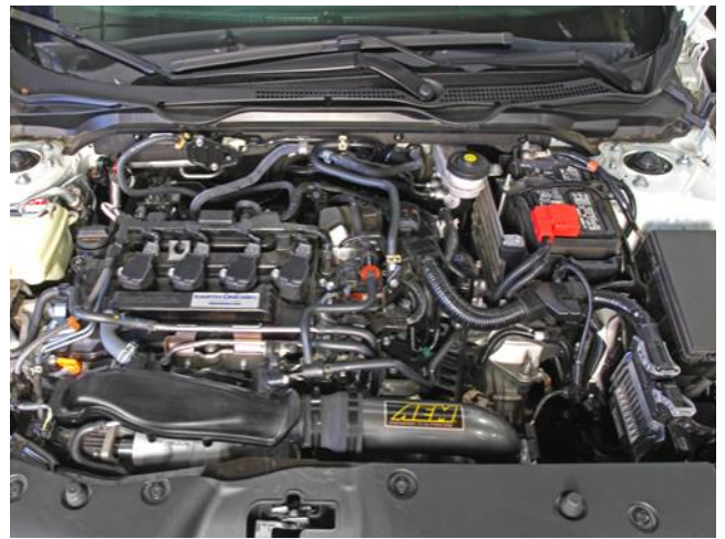
AEM INTAKE INSTALLED
