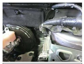
c. Thread the male-to-male rubber isolator mount to the underside of the air box mount as shown.
