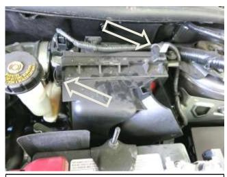
c. Unlatch the two clips holding the two halves of the air box together and remove the front section and air box by tilting it towards the front of the car and lifting it up and out.
