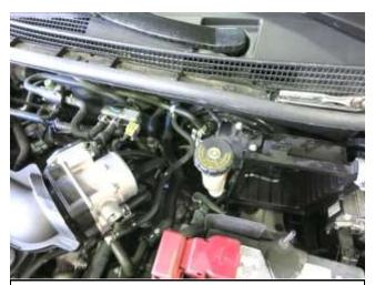
h. Remove the stock rubber air duct first, then remove the remaining section of air box by pulling it up and out of the engine bay.
