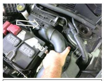
b. Remove the plastic air duct from the stock air box by pulling it straight up while lifting the tab where the arrow is pointing.
