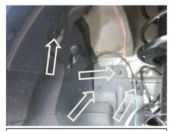
I. Remove the four pop outs shown in the inner fender well area.
