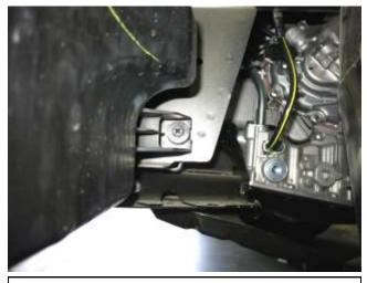
n. Lower the plastic fender liner to access the lower bolt securing the resonator and remove it.
