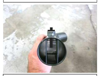
g. Quickly install the air straightener into the long end of the AEM lower intake tube aligning the vanes with the MAF sensor as shown. Refer to the exploded view for clarification.
