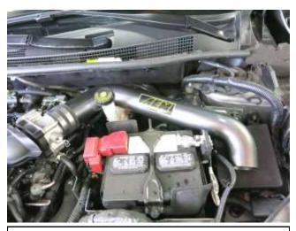
d. Install the AEM upper intake tube as shown and secure the bracket to the isolator using the nut and washer provided.
