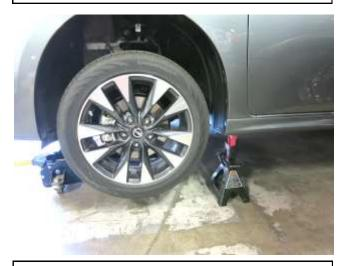
n. Torque all remaining hose clamps to 30 in-lbs, reinstall the engine cover, reassemble the fender liner, install wheel and torque lug nuts, and lower the vehicle.
