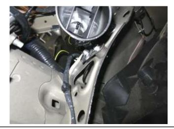
j. 2016 and newer models will require the use of the stainless steel offset bracket as shown. On all models secure the Intake tube bracket with the bolt and washer to the isolator. Note: the wiring harness that runs beneath the tube may need to be loosened and adjusted to fit properly.
