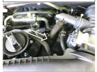
g. Using pliers, release the pressure on the spring clamp holding the vent hose to the engine and disconnect the vent hose from the engine. The two spring clamps will be reused in step 3m.
