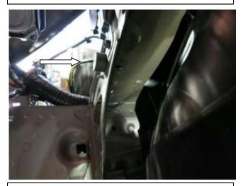
h. On 2015 and earlier models, Install the female to male rubber isolated onto the inner fender as shown.
