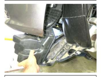
o. Lower the plastic resonator out of the car as shown.Note: Do not discard any of your stock equipment.
