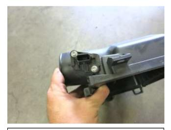
p. Remove the MAF sensor from the stock air box. Note: These screws will be reused in step 3a.
