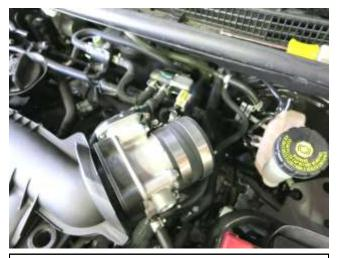
b. Install the provided coupler and hose clamps onto the throttle body. Torque the throttle body side hose clamp to 30 in-lbs at this time.
