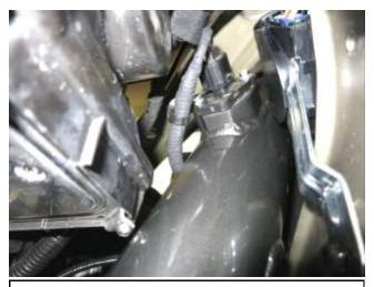
I. Route the MAF harness down to the MAF sensor and connect it as shown.
