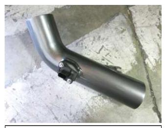
a. Install the MAF sensor into the AEM lower intake tube using the screws removed in step 2p.
