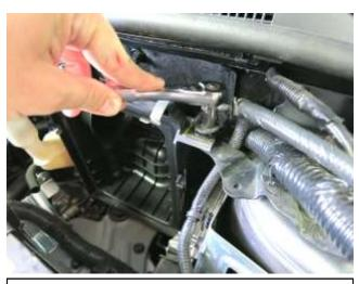
d. Unbolt the other section of the air box as shown.
