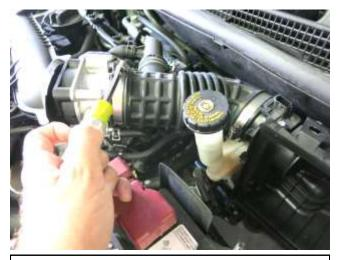
f. Loosen the hose clamps on the throttle body and air box.
