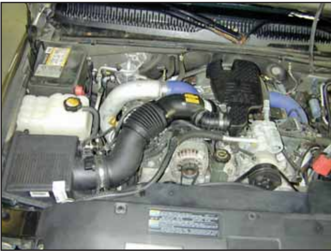
Factory air box system installed
