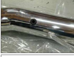
c. Install the rubber grommet into the hole in the intake pipe as shown.
