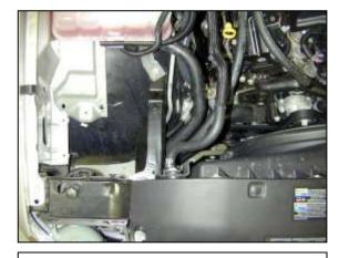
g. Stock airbox system removed from the vehicle.
