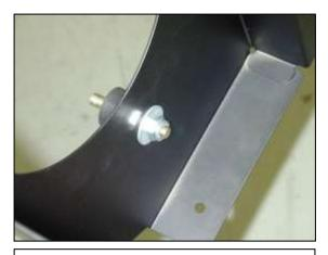
b. Install the supplied rubber mount onto the heat shield as shown using one washer and one nylok nut. Do not fully tighten. It is helpful to run both supplied nylok nuts down the threads once before assembly to make installation easier.
