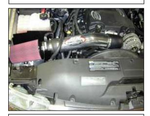
AEM® intake system installed
