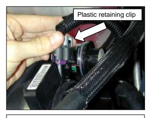
c. Pull back the plastic retaining clip and disconnect the MAF sensor wire harness connector.
