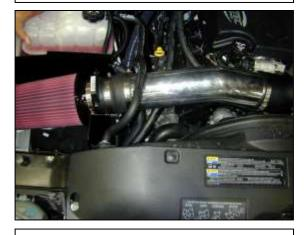
j. Attach the air filter assembly to the intake pipe by sliding the silicone coupler over the intake pipe end. Secure with a supplied #64 hose clamp. Ensure that the air filter does not make contact with any part of the vehicle.
