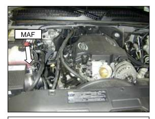
b. Loosen the hose clamp on the rubber elbow attached to the throttle body. Loosen the hose clamp on the MAF sensor and remove the stock plastic intake pipe.
