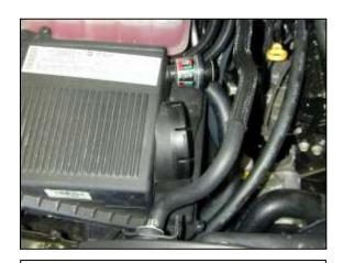
d. Loosen the hose clamp securing the MAF sensor to the stock air filter housing and remove the MAF sensor. Be careful not to damage the sensor!
