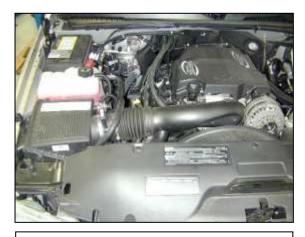
a. Factory airbox system installed.
