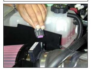
k. Rotate the MAF sensor so the plug is facing up as shown. Plug in the MAF sensor harness as shown. Use the zip tie to secure the harness out of the way and trim the excess.
