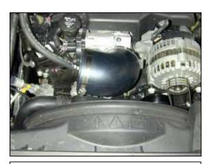
d. Install the supplied rubber elbow onto the throttle body using two #64 hose clamps. Do not fully tighten.
