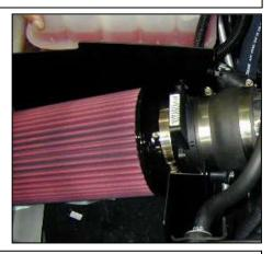
i. Securely attach the air filter to the MAF sensor using the supplied hose clamp (inlet side has the mesh screen). Securely attach the silicone coupler to the other side of the MAF sensor using the # 56 hose clamp.
