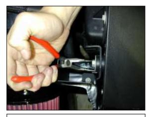
I. Use a pair of pliers and compress the clamp holding the coolant reservoir hose to the radiator. While compressed, rotate the hose up and away from the intake pipe.
