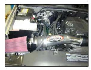
o. Tighten the hose clamps at the throttle body and silicone couplers. Tighten the nut on the mounting bracket. Re-adjust the intake pipe if necessary. Install rubber edge trim to the top of the heat shield and trim as necessary.
