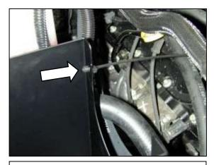
f. Press the supplied zip tie into the heat shield as shown. This will be used to secure the MAF sensor wiring harness.
