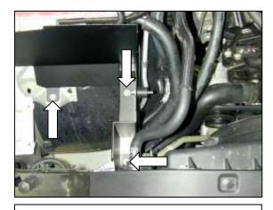
e. Install the heat shield using three of the previously removed stock bolts during step 2(f).
