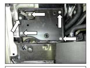
f. Remove the five bolts holding the air filter housing mounting plate to the chassis. Remove the mounting plate and set bolts aside for reuse in a later step.
