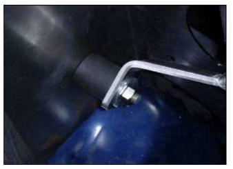
g. Align the intake pipe bracket with the rubber mount on the heat shield. Use the supplied washer and nylok nut to partially secure.
