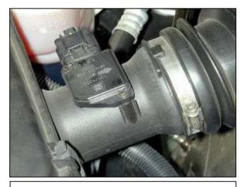
b. Unplug the wire harness from the Mass Air Flow (MAF) sensor. Remove the two screws retaining the MAF sensor and carefully remove the MAF sensor.
