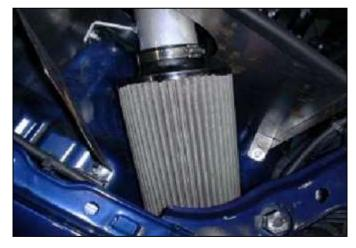
h. Check to be sure that the  $\mathsf{AEM}^{\$}$  air filter is clear from and debris. Attach the air filter to the end of the  $\mathsf{AEM}^{\$}$  intake pipe as shown.
