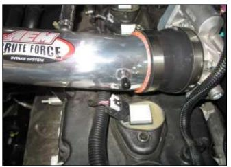
k. For 2006 and newer trucks you will need to plug off the smaller nipple located in the front of the pipe.
