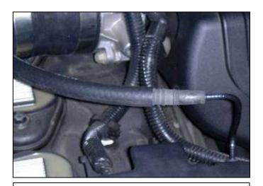
j. Insert the supplied plastic barb fitting into the end of the small breather hose removed in step 2d. Attach the supplied 5/16" hose between the plastic barb fitting and the intake pipe. For the 2006 and newer trucks refer to step 3k.
