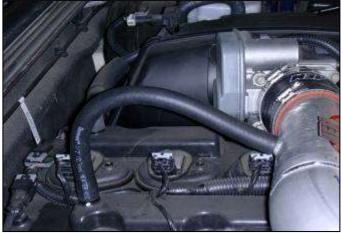
i. Attach the supplied  $\frac{1}{2}$ " hose between the intake pipe and the valve cover as shown. Trim to fit and secure using the supplied hose clamps.
