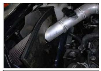
I. Position the AEM<sup>®</sup> intake for best fitment. Be sure that the pipe or any other component is not in contact with any part of the vehicle. Tighten the hose clamps at the throttle body. Tighten the nut on the mounting bracket. Re-adjust pipe if necessary. Re-connect the MAF wire harness.
