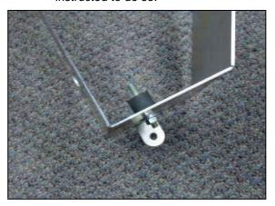
b. Install the supplied rubber mount on to the AEM<sup>®</sup> heat shield using one each of the supplied washers and locknuts.
