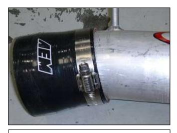
e. Install the reducing coupler on the end of the intake pipe using the #48 hose clamp.
