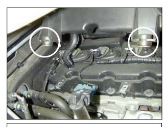
e. Remove the two bolts on the air resonator. Lift the resonator up and remove the breather hose from the valve cover. Remove the small breather hose from the front of the resonator and remove the resonator.
