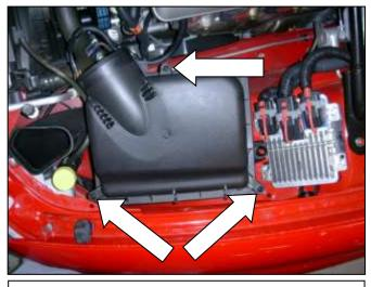
f. Loosen the three screws holding the top of the air filter housing to the filter box and remove the top. Next, remove the air filter from inside the box.
