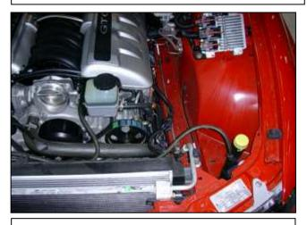
i. Factory air box system removed.
