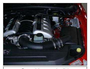
Factory air box system installed
