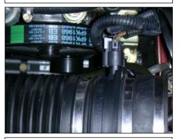
d. Unplug the MAF sensor harness from the MAF sensor and remove the stock inlet air hose and sensor.
