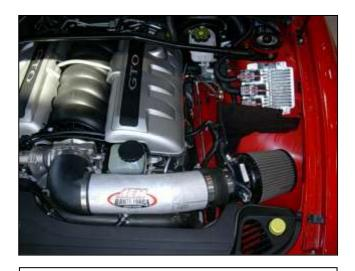
r. Reinstall the radiator shroud and check that the air filter is not touching any part of the vehicle.
