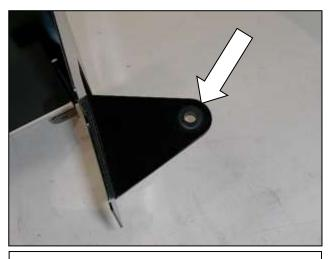
c. Install the rubber grommet into the hole in the heat shield tab as shown.
