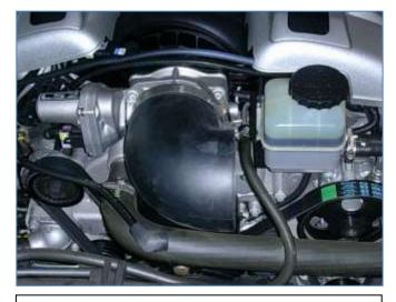
j. Install the long end of the rubber elbow over the throttle body using the supplied #64 hose clamps.
