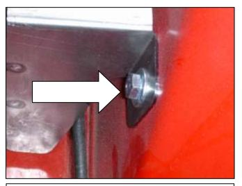
h. Install the M6 bolt with a  $\frac{1}{4}$ " washer through the hole in the tab on the heat shield. Once secured, fully tighten the (2)  $\frac{1}{4}$ " bolts from step 3g.
