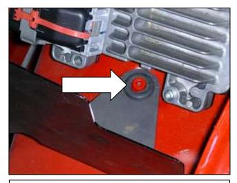
e. Carefully slide heat shield into engine bay. Push rubber grommet installed in previous step over the stud on the strut tower.
