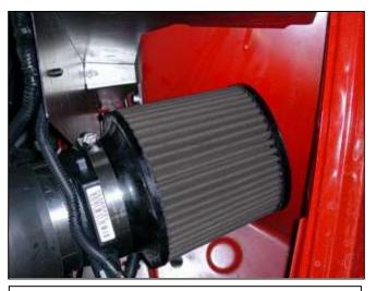
s. Position the AEM<sup>®</sup> intake for best fitment. Be sure that the pipe or any other component is not in contact with any part of the vehicle. Tighten the hose clamps at the throttle body and silicone coupling. Tighten the nut on the mounting bracket. Re-adjust pipe if necessary.
