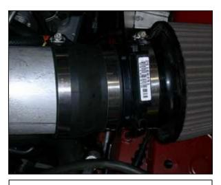
o. Install the MAF sensor and filter into the previously installed reducer coupler. Plug in the MAF sensor and secure the unit using the #56 hose clamp.
