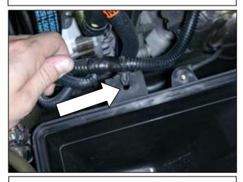
g. Detach the wiring harness air filter housing as shown.
