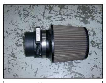
n. Install the AEM® air filter on to the end of the MAF Sensor housing. Push the air filter over the inlet pipe until the stop in the filter is reached; then install one hose clamp to secure the air filter. NOTE: The air filter should be placed on the larger diameter side of the MAF sensor housing.
