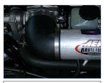
k. Check to be sure the upper intake pipe is clear of any debris. Install the intake pipe by sliding it into the coupler attached to the throttle body.
