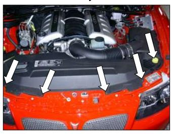
a. Remove the radiator shroud from the front of the vehicle by removing the 5 plastic connectors.
