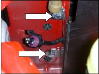
g. Insert the two supplied  $\frac{1}{4}$ " bolts into the holes on steel wall between the radiator and headlight housing. Loosely secure with the supplied  $\frac{1}{4}$ " washers and nylok nuts.
