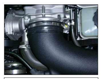
b. Loosen the hose clamp on the inlet hose elbow attached to the throttle body.
