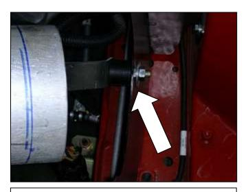
I. Align the intake pipe mounting bracket with the previously installed rubber mount on the heat shield. Use the supplied washer and serrated nut to secure.
