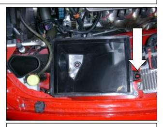
h. The lower air box is held in place with three grommets. To remove it, simply lift up on the box near the ECU.
