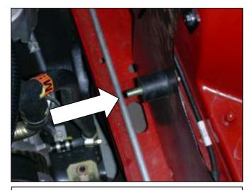
i. Install the supplied rubber mount into the heat shield with the rubber side toward the engine as shown.
