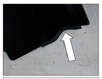
d. Install the rubber edge trim around the cut out where the wire harness will pass through.
