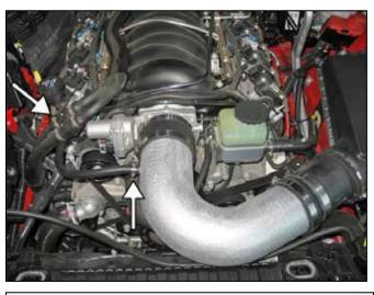
d. Route the breather hose around pulley and under AC lines.
