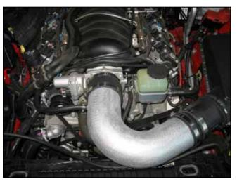
c. Slide coupler over MAF body, then the elbow over the throttle body, align inlet and secure the hose clamps.
