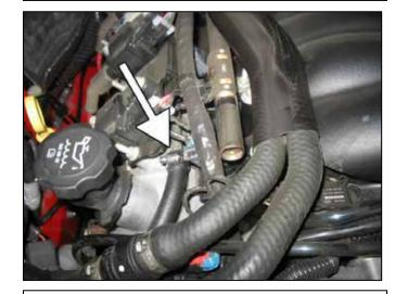
e. Secure the breather hose to the valve cover and re-install the engine cover.
