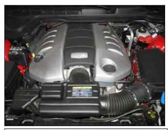
a. Factory air box system installed.
