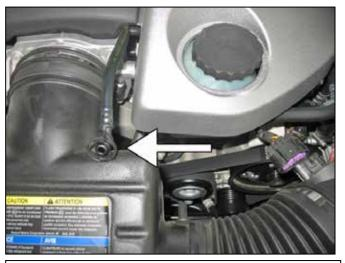
b. Unclip breather hose from resonator chamber
