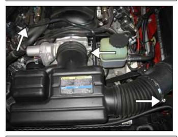
c. Remove engine cover (lift up and pull forward). Loosen hose clamps on the inlet tube at the throttle body and MAF body. Also disconnect and remove the breather hose from the valve cover.
