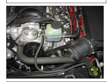
d. Remove the inlet tube.
