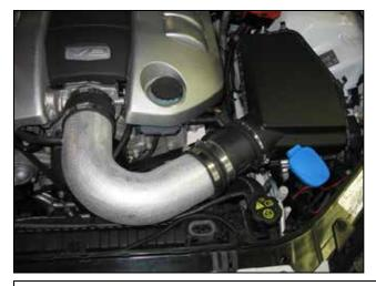
AEM® intake system installed
