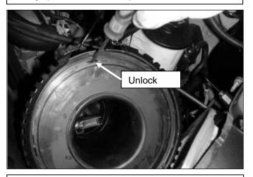
i. Unlock the MAF sensor from its housing.
