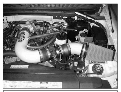
w. Plug the wire harness connector back into the MAF sensor.
