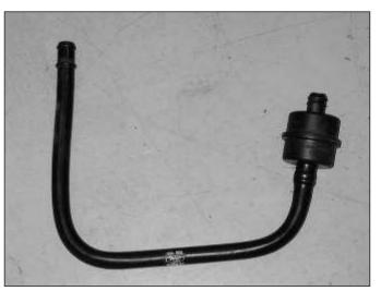
o. Remove this portion of the IAC breather tube from the vehicle. Remove the tube from the check valve, the check valve will be used with the  $\mathsf{AEM}^{\textcircled{\$}}$  intake system.
