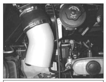
m. Insert the second inlet pipe. The bracket will be inserted underneath the tab on the power steering reservoir.
