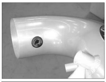
c. Insert the grommet into the upper inlet pipe.
