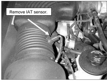
f. Remove the IAT sensor from the air inlet tube.
