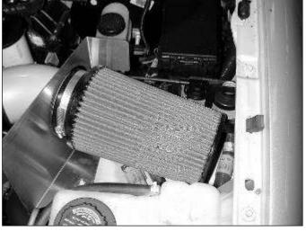
v. Attach the air filter to the inlet pipe. Check for clearance and secure the air filter.
