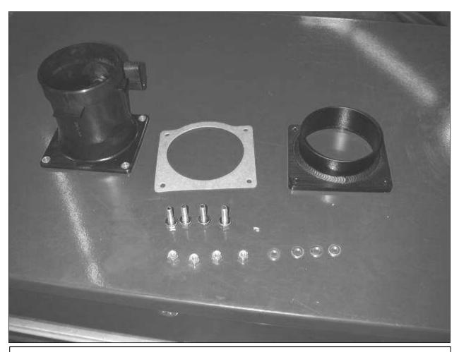
h. The new MAF sensor assembly will contain the above hardware. 1 MAF sensor, 1 gasket, 4 M6x20 bolts, 4 nylok nuts, 4 M6 washers and the MAF sensor adapter.
