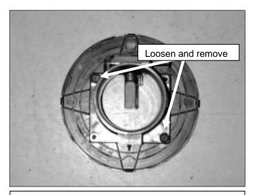
f. Loosen and remove the two bolts on the stock MAF assembly.
