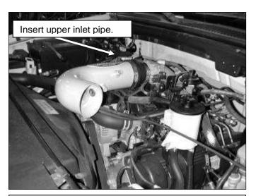
d. Insert the upper inlet pipe into the reducer coupler on the throttle body and secure with a hose clamp.
