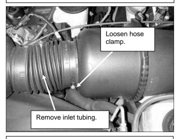
g. Loosen the hose clamp and remove the inlet tubing up to the throttle body.
