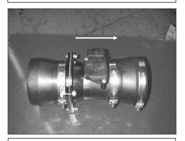
k. Attach the reducer couplers and 3 hose clamps to the MAF assembly as shown. The flow arrow is pointed to the right on the MAF sensor.
