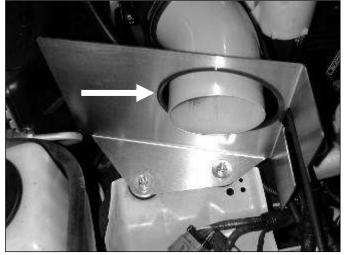
p. Attach rubber edge trim as shown. Secure the heat shield with the supplied washer and Nylock nuts. Make sure the heat shield clears the A/C line on the left and the cruise control on the right.
