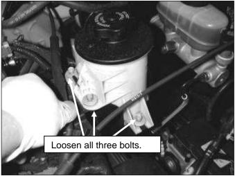
e. Loosen the three bolts securing the power steering reservoir.
