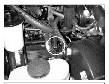
u. Attach the other end of the crankcase breather tube to the nipple of the crankcase and secure.
