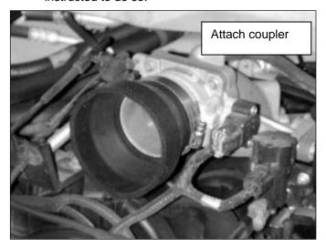
b. Attach the reducer coupler and hose clamp to the throttle body.
