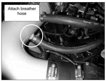
t. Attach crankcase breather tube and secure to the lower nipple on the inlet pipe.
