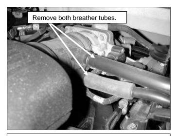
e. Remove the IAC and crankcase breather tubes from the upper air inlet tube.
