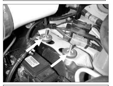
o. Insert the bolt and washer from underneath the rubber grommet. Insert the heat shield spacer and secure with the nut.
