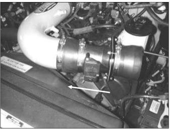
I. Attach MAF assembly to the upper inlet pipe, the flow arrow on the MAF sensor should be pointing to the upper inlet pipe.
