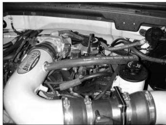
r. Secure IAC's breather hose to the upper nipple on the inlet pipe.
