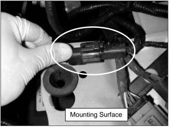
n. Remove the clip for the MAF sensor harness connector that secures it to the mounting surface. Ensure the mounting surface is level so the heat shield can be properly mounted.
