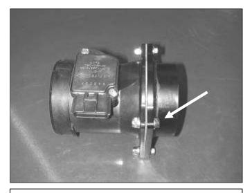
i. Assemble the MAF sensor and hardware like the assembly in the image above. The order is nylok nut, washer, MAF sensor, gasket, MAF sensor adapter, and bolt head.
