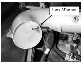
j. Insert the IAT sensor into the grommet in the upper inlet pipe.
