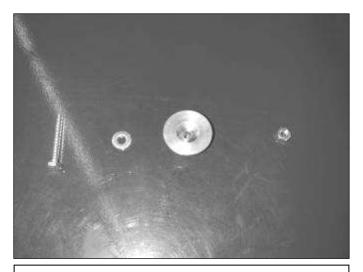
n. This is the hardware that attaches the heat shield to the mounting surface. 1  $\frac{1}{4}$ -20 bolt,  $\frac{1}{4}$ " washer, heat shield spacer, and  $\frac{1}{4}$ -20 nut.
