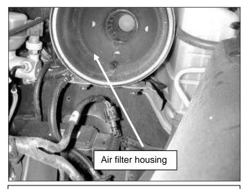
m. Remove the air filter housing.
