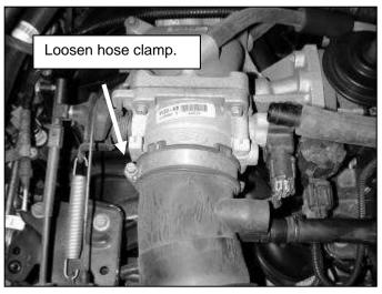
d. Once the throttle body cover is removed, loosen the hose clamp securing the inlet tube to the throttle body.
