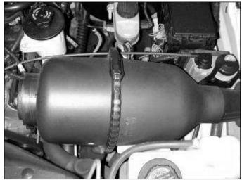
h. Unclasp the latch for the air filter and MAF sensor.
