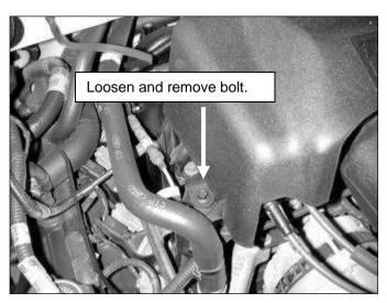
b. Loosen and remove the bolt on the left side of the throttle body cover.
