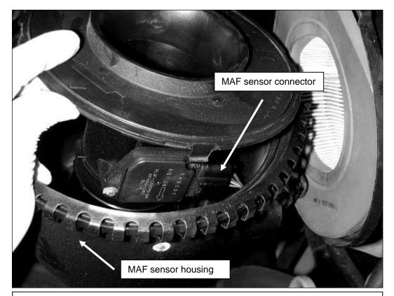
j. With the assembly open, locate the MAF sensor. Disconnect the MAF sensor and pull the connector from the housing. The MAF sensor housing will not be reused.
