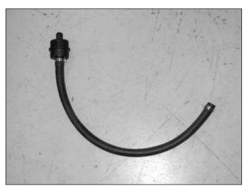
${\bf q}.$  Attach breather hose for the IAC and secure it to the check valve.
