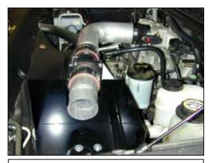
q. Align the both inlet pipes along with the MAF sensor assembly to the bracket on the heat shield.
