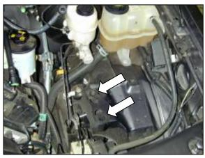
b. Remove rubber grommets left by the filter element housing.
