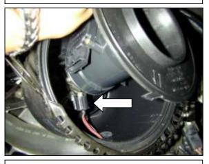
g. Disconnect the MAF sensor connector from the MAF sensor. *Careful not to damage MAF sensor harness.*
