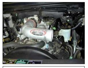
j. Insert the upper inlet pipe into the coupler and secure.
