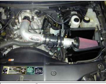
AEM<sup>®</sup> intake system installed
