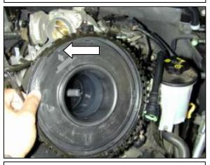
f. Gently pry open the housing at the any one of the tabs. *Careful not to damage the MAF* sensor.
