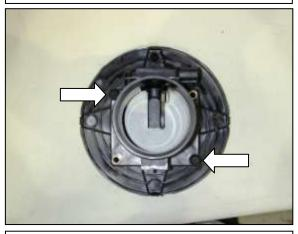
h. Loosen and remove the two screws holding the MAF sensor.
