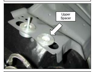
d. On the left is a fully assembled anchor for the heat shield. On the right, insert the upper spacer into the stock housing mounting surface.
