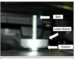
c. Assemble the following bolt, washer and lower spacer.
