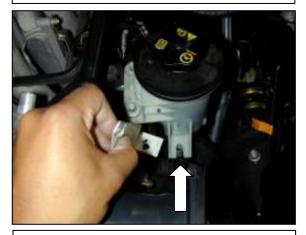
n. Remove the front bolt that secures the power steering fluid reservoir. Loosen the other two bolts. Place the MAF sensor bracket tab under the front tab of the power steering fluid reservoir. Secure mounting position, but do not fully tighten.
