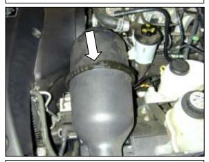
e. Unclasp the clip holding the air filter element casing together.
