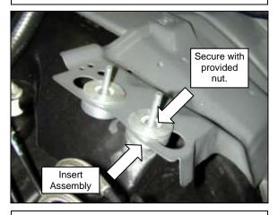
e. Insert the assembly from *Step 3c* into the upper spacer from underneath. Secure with provided nut.
