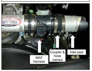
p. Re-attach the MAF sensor connector. Attach the last coupler to the MAF sensor assembly and secure with hose clamps. Insert the second inlet pipe and align with rubber mount.
