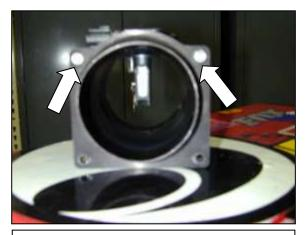
I. Attach the MAF sensor adapter to the MAF sensor. Secure the adapter with the M6 bolt and nylok nut only to the holes located nearest the sensor.
