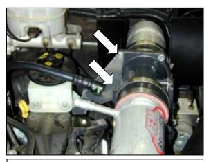
r. Secure the MAF sensor bracket to the remaining two holes on the assembly. Realign to the rubber mount and secure rubber mount to the pipe bracket. Check clearance through the heat shield.
