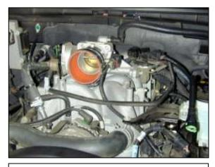
i. Attach the reducer coupler to the throttle body and secure with hose clamp #48. The other end should not be tightened.
