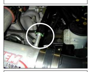
s. Re-attach breather hose. Make sure connector snaps onto the nipple.
