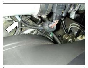
t. Secure MAF wire harness away from the fan with provided zip tie. Failure to do so may damage harness and may result in engine failure.
