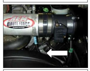
m. Insert the MAF sensor assembly into the coupler. NOTE: Make note of the air flow direction.
