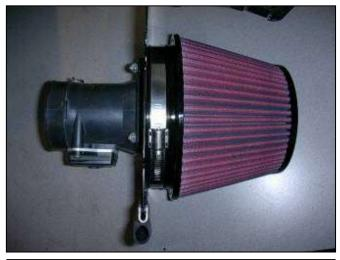
i. Install the  $\mathsf{AEM}^{\text{(8)}}$  air filter onto the MAF sensor adapter as shown.
