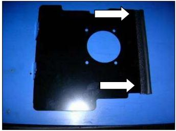
c. Install the gasket material to the top of the heat shield.
