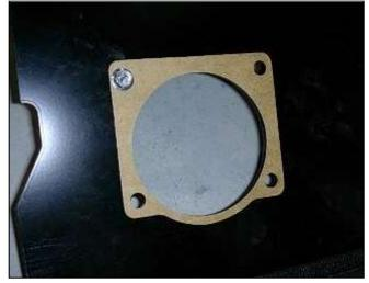
g. Place one of the supplied gaskets onto each side of the large hole in the heat shield.
