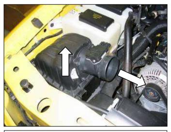
e. Remove the inlet pipe. Remove the air box by first pulling it up and then towards the center of the vehicle.
