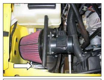
j. Place the heat shield/air filter/MAF sensor in the engine bay. Secure it to the chassis with the original bolts.
