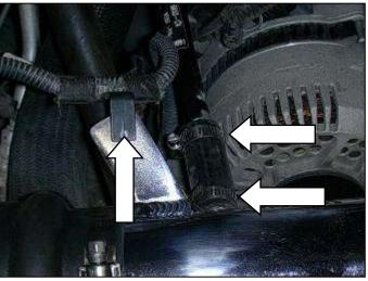
m. Secure the breather hose to the inlet pipe with the supplied hose and hose clamps. Install the MAF sensor wiring harness support into the tab on the pipe.
