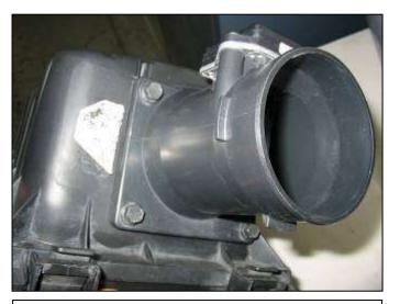
f. Remove the MAF sensor from the air box.
