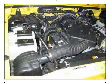
a. Factory air box system installed.
