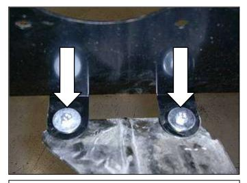
d. Secure the air box support plate to the heat shield with the supplied hardware. Refer to step 'e'.
