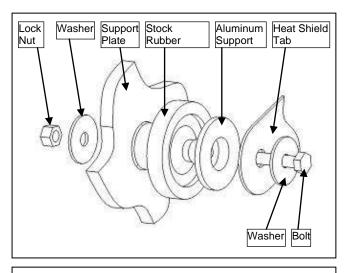
e. Proper heat shield hardware alignment.
