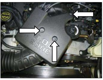
b. Remove the three screws that secure the throttle body cover. Remove the throttle body cover.
