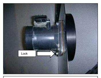
h. Secure the MAF sensor and MAF sensor adapter to the heat shield with the supplied bolts and lock nuts.
