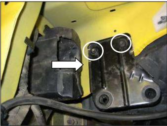
f. Remove the silencer behind the headlight. Remove the air box support plate.
