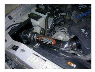
n. Plug the wiring harness into the MAF sensor. Install the throttle body cover.
