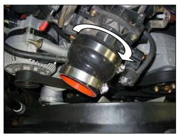
b. Place coupler over the throttle body as shown. Align the worm screw of the large hose clamp <u>AWAY</u> from the throttle body cable pulley. Tighten the large clamp.
