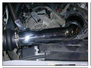
I. Place the inlet pipe in the engine bay as shown.
