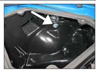
k. Secure the airbox to the vehicle's frame using the supplied M6 bolt (# 1-2038) and washer (# 08160).
