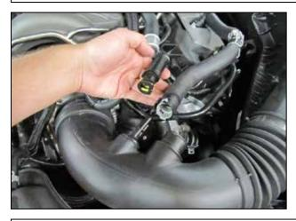
g. Release the crankcase vent tube from the nipple. Slide the gray clip to the side and pull on the connector to release it. On auto. trans. vehicles, also release the smaller vent tube by squeezing the yellow clip.
