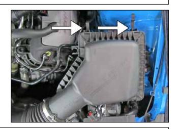
j. Release the two airbox clips as shown.
