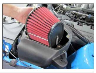
s. Attach a (#9456) hose clamp onto the air filter and lower it into the airbox as shown. Feed the 5/32" hose up through the grommet from inside the airbox.
