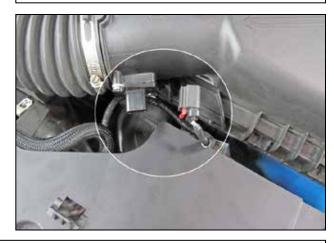
d. Unplug the MAF sensor. First pull back on the red latch, then squeeze to release the connector.
