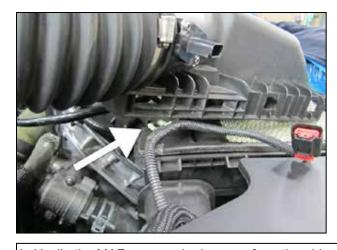
k. Unclip the MAF sensor wire harness from the airbox lid.
