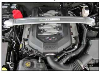
a. Loosen and remove the 4 nuts securing the strut brace.
