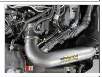
o. Connect the sound tube to the AEM® intake pipe and secure it in place with the OEM spring clamp.
