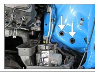
g. Install the two larger grommets (#784645) into the holes in the inner fender area as shown.
