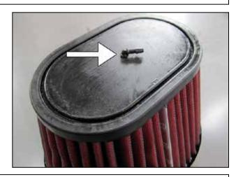
q. Insert the 90 degree plastic connector into the hole located on the air filter top.
