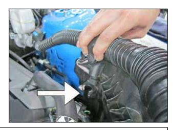
f. Lift up on the rubber support to release it from the OEM airbox.
