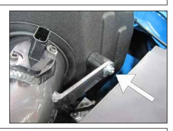
w. Secure the pipe bracket to the rubber mount with a supplied M6 nut (# 444.460.04) and washer (#08160).
