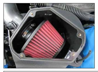
t. Install the air filter onto the end of the AEM® intake pipe and position the filter as shown. Make sure that the pipe is bottomed out on the stops within the air filter. Once proper fitment of the air filter is achieved, secure the (#9456) hose clamp.
