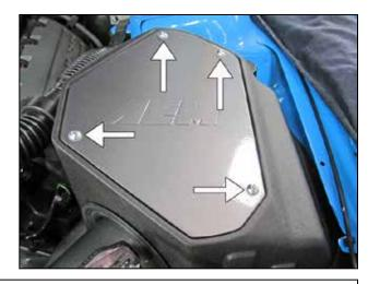
y. Install the AEM® airbox lid using the 4 supplied M6 button head bolts (# 1-112) and nylon washers (#1-3001).
