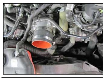
c. Install the 3.5" coupler and two (#9456) hose clamps onto the throttle body. Slide the coupler all the way onto the throttle body, position the hose clamps as shown, and tighten the throttle body-side hose clamp.
