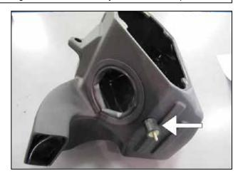
e. Install the rubber mount into the AEM® airbox as shown. Thread the short stud of the rubber mount into the airbox's threaded hole; hand tighten.
