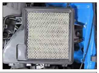
I. Remove the inlet tube from the throttle body and lift the airbox lid off of the lower airbox. Remove the airbox and inlet tube assembly.
