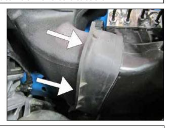
i. Make sure that the large rectangular inlet engages the OEM air scoop.
