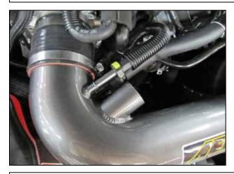
n. Connect the OEM vent tube(s) to the AEM® intake pipe by firmly pressing the connector onto the respective nipple until it 'clicks' into place. On manual trans. vehicles, cap the smaller nipple with the supplied vac. cap. (#8-101).
