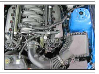
h. Position the sound tube and crankcase vent tube out of the way as shown.
