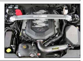
aa. Reinstall the strut brace and tighten all 4 nuts.
