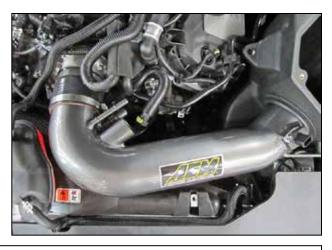
m. Insert the end of the AEM® intake pipe into the throttle body coupler as shown.
