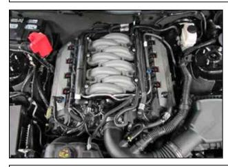
c. Remove the engine cover by lifting up on it from the front and releasing the 4 snap clips.
