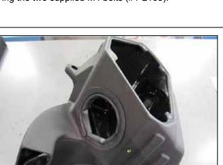
d. Install the rubber edge trim onto the AEM® airbox's round inlet hole as shown. If necessary, trim the edge trim for proper fitment.
