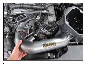
I. Install the AEM® intake pipe as shown. Make sure that the bracket engages the stud on the rubber mount.
