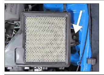
m. Remove the M6 bolt securing the lower airbox, then remove the lower airbox.
