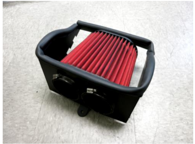
d. Install the AEM® filter into the heat shield with the provided hose clamps.
