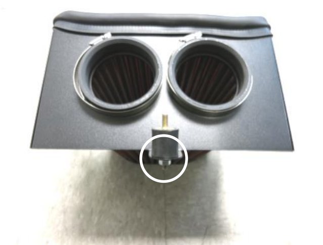
e. With the provided hardware, install the rubber mount/washer/nut onto the heat shield tab.
