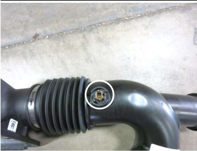
g. Remove the air intake temperature sensor from the stock intake tube. Note: This will be reused in step 3b.
