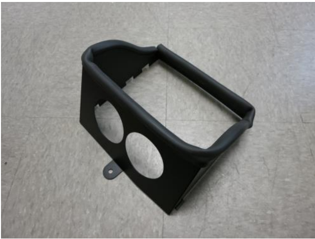
c. Install the provided edge trim onto the heat shield as shown. Note: Trimming the edge trim maybe necessary.
