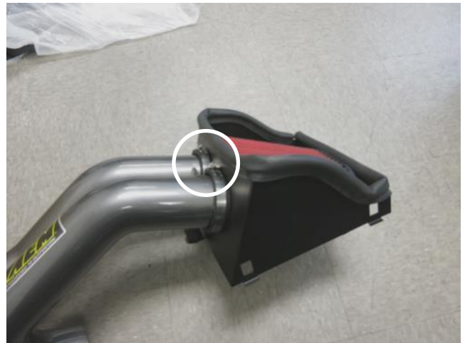
f. Install the AEM® intake tube into the AEM® air filter while aligning the rubber mount with the bracket on the intake tube. Tighten the hose clamps on the filter.
