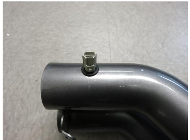
b. Install the air temperature sensor that was removed in step 2g into the AEM® intake tube.
