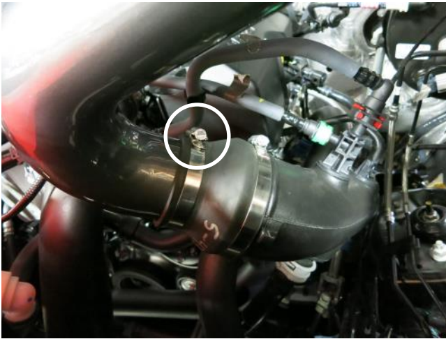
k. Align the AEM® intake tube with the step coupler that was previously installed in step 3h. Tighten the hose clamp circled at this time.
