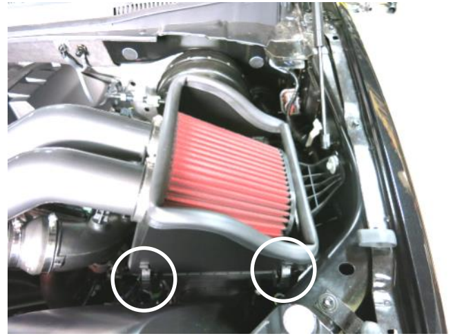
j. Install the assembled AEM® intake tube and heat shield into the vehicle. Align the heat shield into the lower air box and latch the clips to secure it in place.
