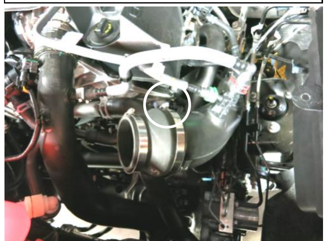
h. Install the step coupler with the provided hose clamps onto the lower intake tube as shown. Tighten hose clamp circled.
