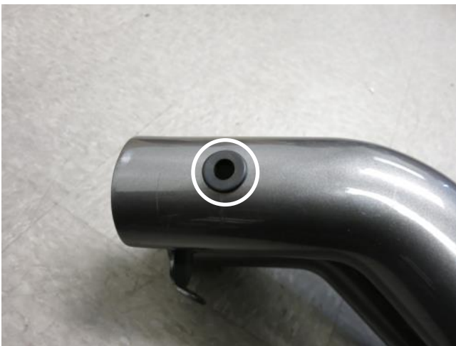
a. Install the provided grommet into the AEM® intake tube.
