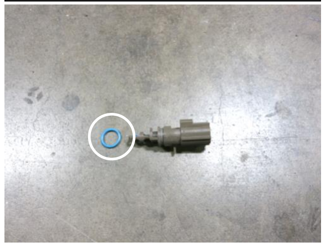
h. Remove the O-ring from air temperature sensor. Note: The O-ring will not be reused.
