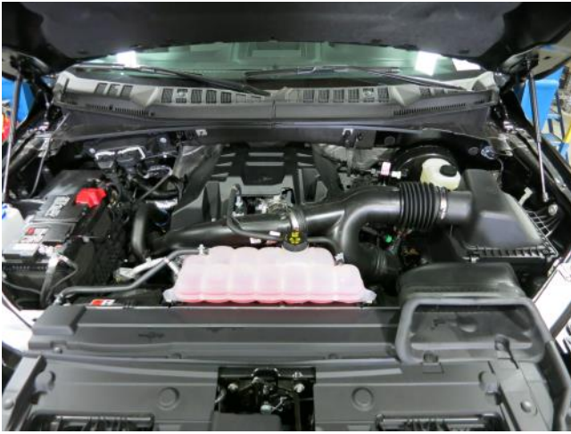
STOCK INTAKE INSTALLED
