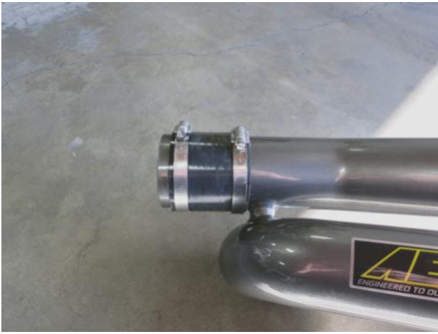
i. Install the straight coupler with hose clamps onto the AEM® tube. Note: Use soap and water to allow the coupler to slide on the intake tube.
