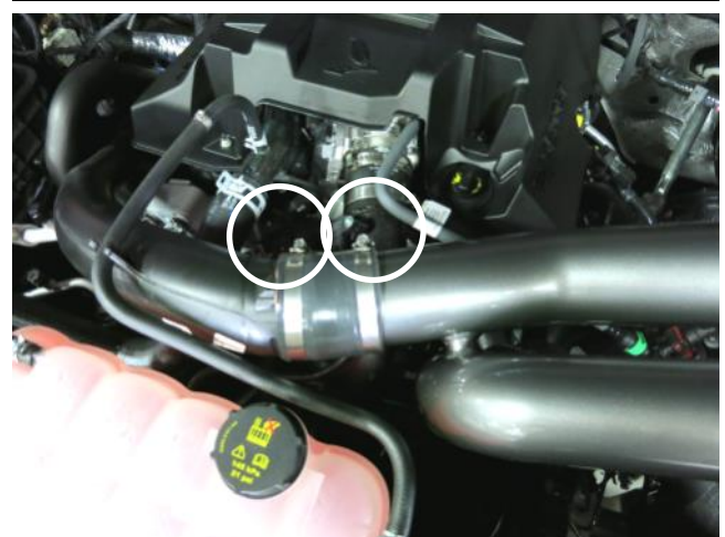
l. Install the straight coupler with hose clamps onto the stock upper intake tube. Tighten both hose clamps at this time.
