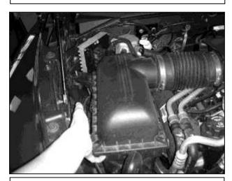
h. Gently pull the airbox out of the rubber grommets and remove the entire intake system from the engine bay.
