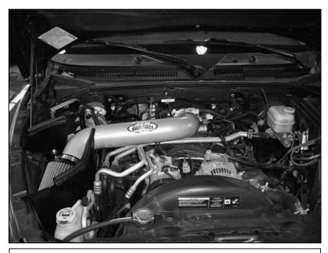
AEM intake system installed
