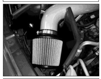
n. Insert the air filter onto the end of the intake pipe. Secure with the supplied hose clamp.
