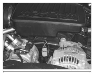
e. Remove the two resonator bolts.
