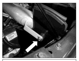
k. Be sure that the pipe bracket is in a flat position over the rubber mount. Loosely install the supplied washer and nut over the bracket.
