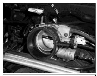
i. Place the #52 hose clamp on the smaller end of the reducer coupler. Attach the smaller end of the reducer coupler to the throttle body with the IAT sensor directed to the right of the throttle body.
