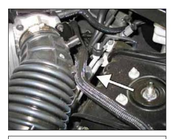
e. Remove the coolant line from the air tube.
