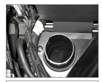
e. Insert the push-in clip on the heat shield base.
