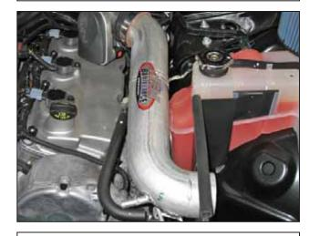
i. Insert the intake pipe as shown. Align the intake pipe bracket with the rubber mount.
