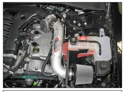
AEM® intake system installed
