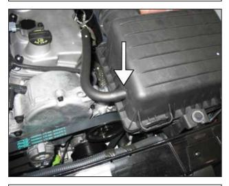
c. Remove the PCV breather tube from the air box.
