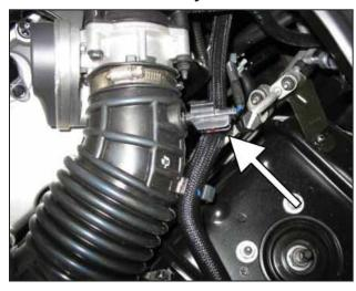
a. Disconnect the inlet air temperature (IAT) sensor connector.
