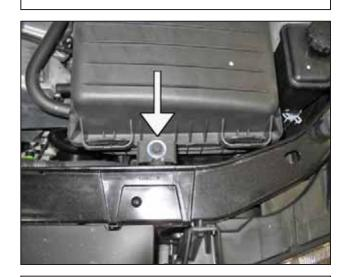
d. Loosen and remove the air box mounting screw. This screw will be reused.
