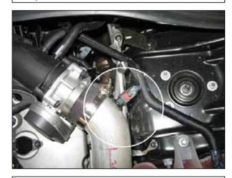
m. Insert the grommet for the IAT sensor into the intake pipe. Insert the IAT sensor and reattach the IAT sensor harness connector that was disconnected in step 2a. Secure the intake pipe to the throttle body coupler.
