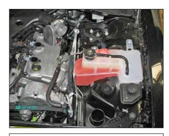
f. Remove the air box assembly from the engine bay.
