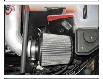
I. Attach the AEM<sup>®</sup> Dryflow<sup>™</sup> air filter. Check for clearance around the rubber edge trim and secure.
