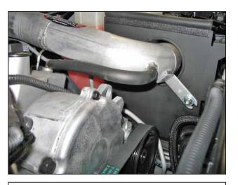
k. Reattach the PCV breather hose to the breather nipple on the intake pipe. Secure with a hose clamp.
