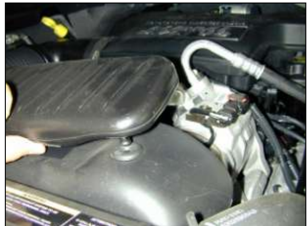
d. Pull the front resonator free of the mounting grommet on the fan shroud. Remove the air cleaner housing/intake tube/front resonator assembly from the engine bay.
