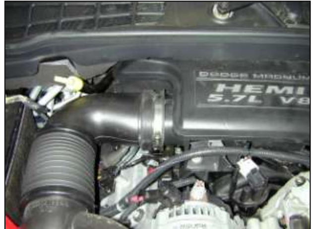
b. Loosen the hose clamp at the intake air resonator. Pull the intake hose clear of the intake resonator.
