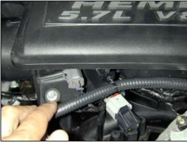
e. Unplug the IAT sensor connector and pull the wire harness clip free from the mount on the front of the resonator.
