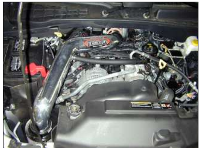
AEM ® intake system installed
