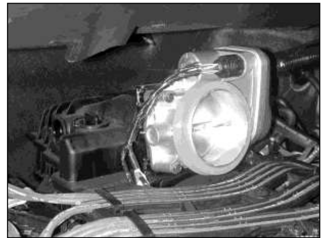
h. Remove the orange rubber gasket from the throttle body.
