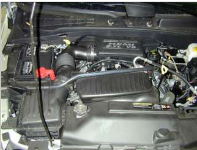
Factory air box system installed
