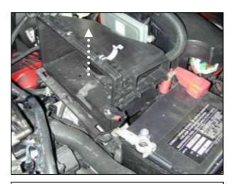
h. Pull up on the other half of the air box and remove the air box.
