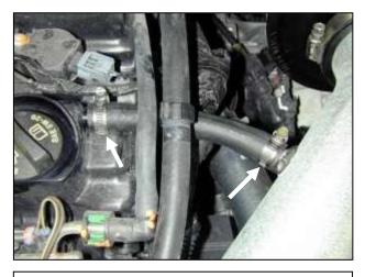
I. Attach the breather hose as shown to the inlet pipe and to the crank case vent. Secure with hose clamps.
