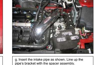
pipe's bracket with the spacer assembly.
