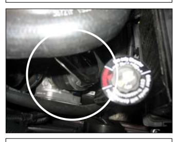
h. Insert the other end of the inlet pipe into the coupler at the throttle body. Realign the bracket and secure the hose clamp.
