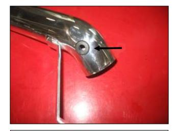
c. Insert the supplied grommet for the IAT sensor into the inlet pipe.
