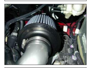
i. Attach the air filter. Check for clearance and secure hose clamp.
