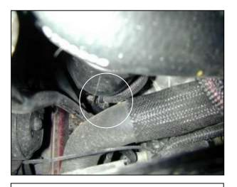
f. Remove the tree mount zip tie from the inlet tubing. Remove the inlet tube and the IAT sensor.
