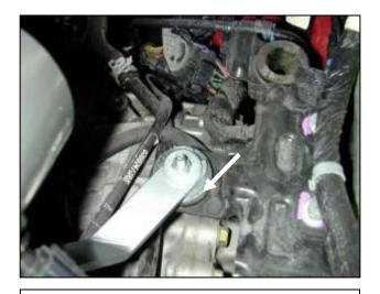
j. Check for clearance of the inlet pipe around the coolant hose. Tighten the bracket with a washer and a lock nut.
