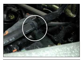
m. Secure both breather hoses with the factory clip (*If equipped*). Reinstall the engine cover.
