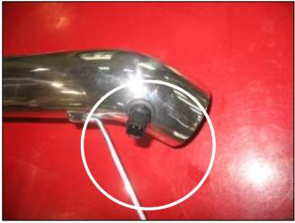
f. Insert the IAT sensor into the grommet from step 3c.
