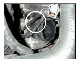
b. Attach the reducer coupler to the throttle body. Secure with the 2.5" hose clamp. Loosely attach the hose clamp to the other side of the coupler.
