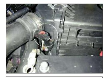
e. Remove the intake air temperature (IAT) sensor harness connector. Pull the tab out and then depress the clip to remove.
