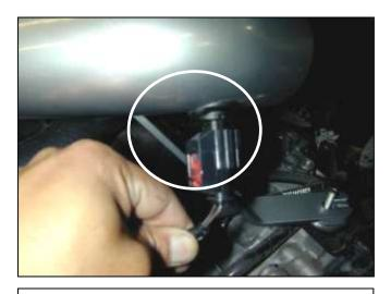
k. Reattach the IAT sensor wire harness connector. Check for clearance around the negative battery terminal.
