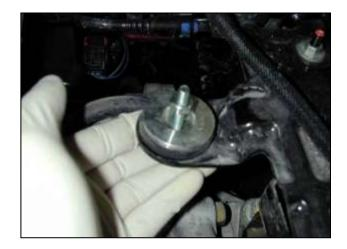
e. Insert the spacer over the bolt. Secure the threaded bolt with the provided nut. Center the spacer in the grommet and tighten.
