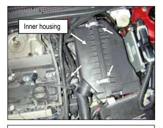
g. Disconnect the crank case breather hose from the valve cover. The other end will be connected to the air box. Unclasp the air box and remove the inner housing, air filter and breather hose.
