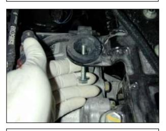
d. Insert the threaded bolt and a ¼" washer up through the air box mount grommet.
