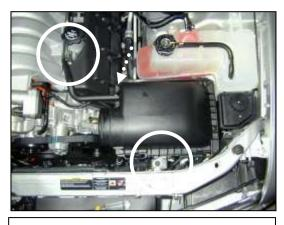
e. Disconnect the crank case breather tube at the intake manifold. Loosen and remove the air box mounting bolt. Remove the air box by pulling straight up.
