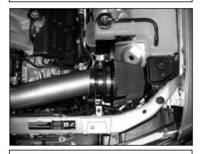
n. Attach the air filter assembly to the coupler and secure with hose clamps.
