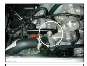
f. Loosen and remove the nut. Remove bracket and reinstall the nut.
