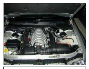
a. Stock air box system installed.
