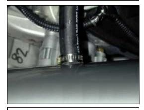
o. Attach the new crank case breather hose to the inlet pipe. Tighten provided hose clamp to secure.
