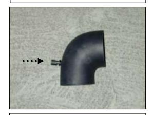
i. Insert the IAT sensor into the coupler. Be careful not to damage the sensor.
