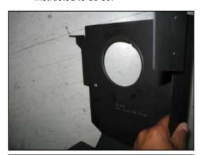
b. Attach the rubber edge trim to the inlet pipe opening on the heat shield. Trim excess.
