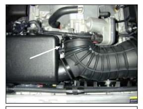
b. Loosen the throttle body hose clamp.
