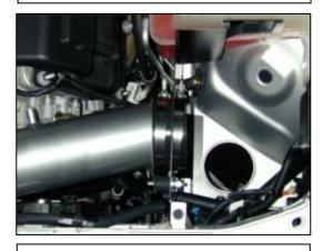
m. Attach the coupler and hose clamps to intake pipe and then secure.
