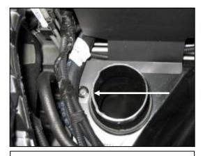
e. Insert the push-in clip on the heat shield base to secure.
