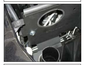
h. Secure the rubber mount with the M8 washer and nut.
