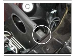
f. Secure the remaining tab with the factory screw.
