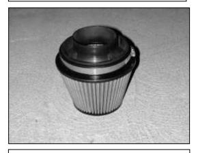
I. Insert the adapter into the filter element. Secure with hose clamp.
