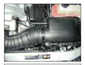
d. Loosen the inlet tube hose clamp. Remove the inlet tube.
