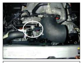
j. Attach the smaller end of the coupler to the throttle body and secure with provided hose clamp as shown. Reconnect the IAT sensor wire harness connector and lock in place.
