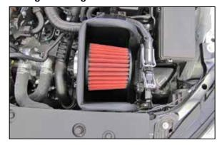
8. Set the AEM® air filter into the heat shield assembly.
