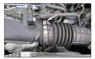
3. Loosen the hose clamp that secures the intake hose to the turbo inlet.
