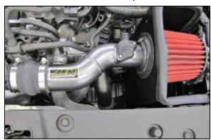
11. Install the AEM® intake tube through the heat shield and into the AEM® air filter, then install onto the turbo inlet. Align the tube for best fit and then secure with the provided hose clamp.
