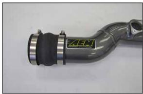
9. Install the provided hump coupler (08487) onto the intake tube and secure with the provided hose clamp.
