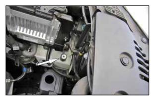
5. Install the rubber mounted stud onto the frame rail where shown.
