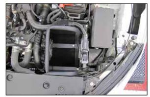
7. Install the heat shield assembly onto the frame rail and secure with the provided hardware. NOTE: The heat shield will bolt to the rubber mounted stud and to the factory rear air filter housing mounting location.
